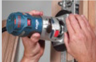
Route Hinge Mortises
