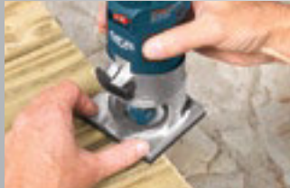
Round Off Deck Planks & Rails
