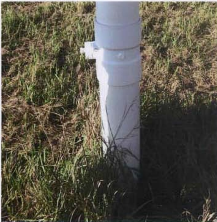
Landfill Cap, Facing North, Monitoring Well Nest MW-2S, MW-2M and MW-2D in Center Cap was recently mowed to facilitate inspection.
