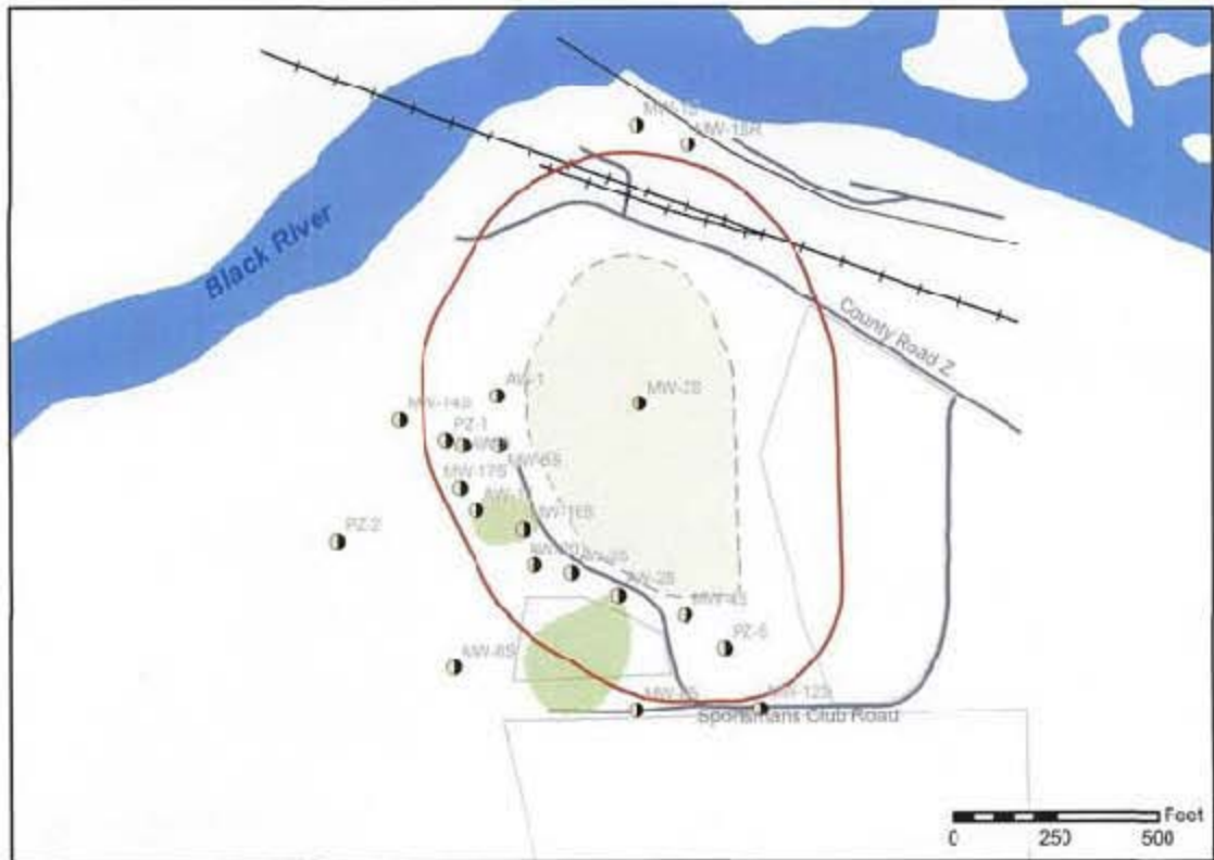
Figure 16 Map of Combined VOC UCL Target Zones for the A) Shallow Wells and B) Medium-Depth Wells
