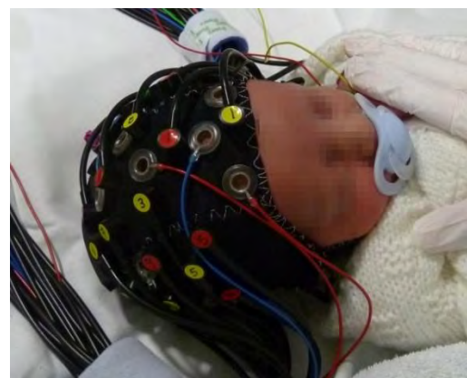
Figure 2. An infant in a soft DOT imaging cap. Prism-coupled fibres will be used to perform fast TR-DOT using this arrangement.
