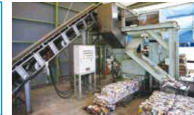
Shigen-Ka-Kun II + Press machine ACP-100-2 (operation capacity: 5 t / day)
