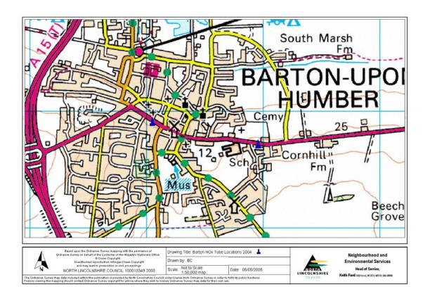
NO<sub>2</sub> diffusion tubes are used to monitor emissions from road traffic. An annual review is conducted which considers data collected over the year and any changes to road traffic flows. Tubes are then relocated as required in accordance with DEFRA Technical Guidance LAQM.TG(03). New locations for 2004 are detailed in Table 10 Section 2.3.1.
