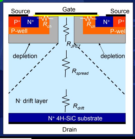
**Pursuing DMOSFET** As Switch From 600V Up To 10kV **DMOSFET** Requirements Low R<sub>on,sp</sub> **Low Conduction Losses High Switching Speed** Low Switching Losses ۲ **Manufacturable High-**• **Yield Design/Process**
