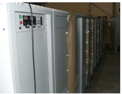
Photograph: a 400-kW current source DC-DC converter
