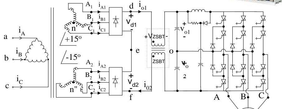
• Possible to use HV - IGBTs with SiC diodes
