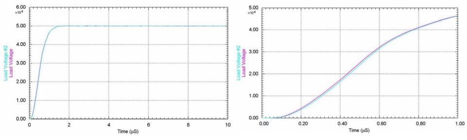
10 & 12 Pulse Output Voltages "Overlay" (2 failed switching assemblies) Slight Change In Rise Time For 10 Pulse vs. 12 Pulse Operation (no significant difference)
