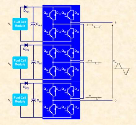
7-level cascaded multilevel inverter
