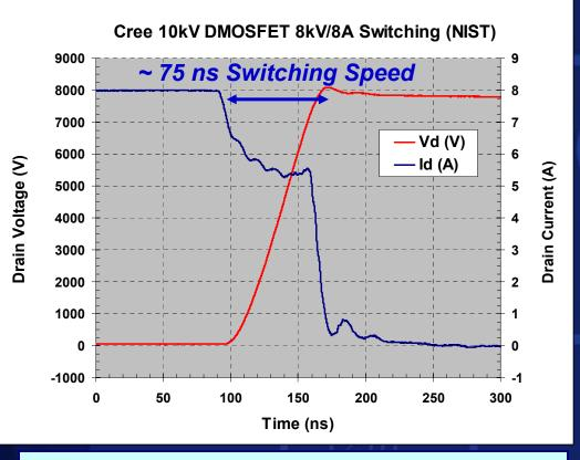
Measured Switching Speed of ~ 75 ns for 10kV SiC DMOSFET at 25°C
