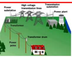
AC won (pre-electronics) •Transformer isolation •Impedance (V) transformation •Grounded Secondary (safety) •AC → DC, easy
