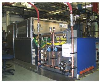
20 KHz, 10 MW Polyphase Pulsed Converter
