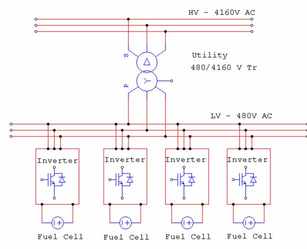
Note: Fuel cells share common fuel supply and control systems, pumps etc. • Each Fuel Cell & its Inverter is rated for say 300kW
