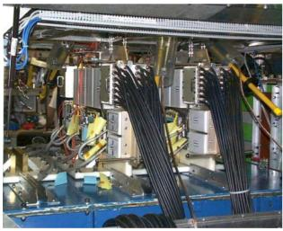
20 KHz IGBT Switching Assemblies
