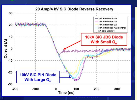
10kV/20A SiC JBS Diode Has Much Smaller Reverse Recovery and Higher Switching Speed Compared to PiN
