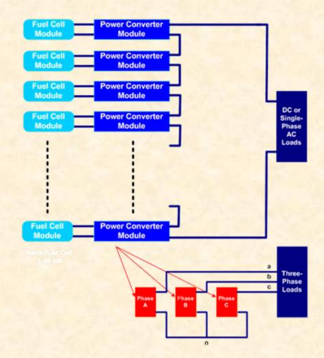
Each power converter module typically consists of a dc/dc voltage regulator and an H-bridge inverter
