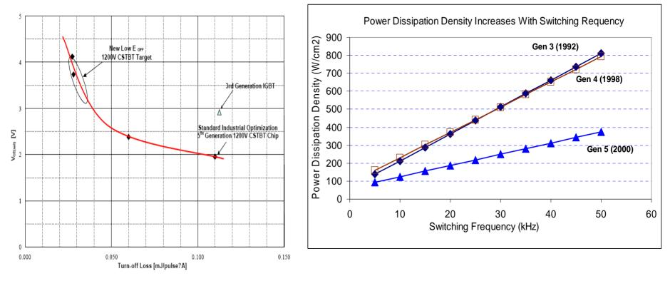
Conduction vs Switching Loss Trade-Off
