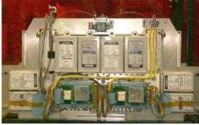
IGBT switch plate assembly (LANL SNS modulator)
