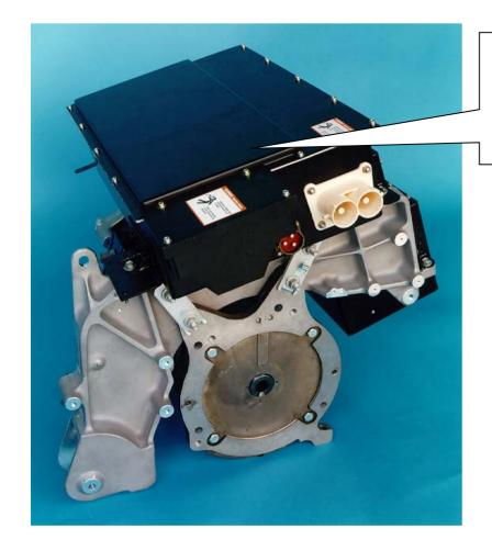
100kW motor drive inverter 1.3 ft<sup>3</sup>, 56lb DC input 320V
