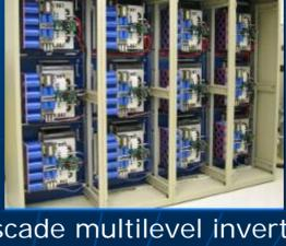
Cascade multilevel inverter Fang Peng, MSU
