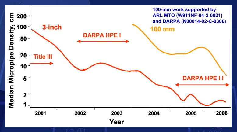
Cree Monthly Median Production SiC Substrate Micropipe Density (MPD)
