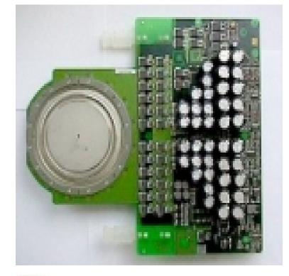
The ACS 1000 is the first drive to use a new power semiconductor switching device called IGCT (Integrated Gate Commutated Thyristor). This advanced, highpower semiconductor approaches the "ideal switch" for mediumvoltage applications. IGCT brings together a versatile new power handling device, the GCT, (Gate Commutated Thyristor) and the device control circuitry in an integrated package.
