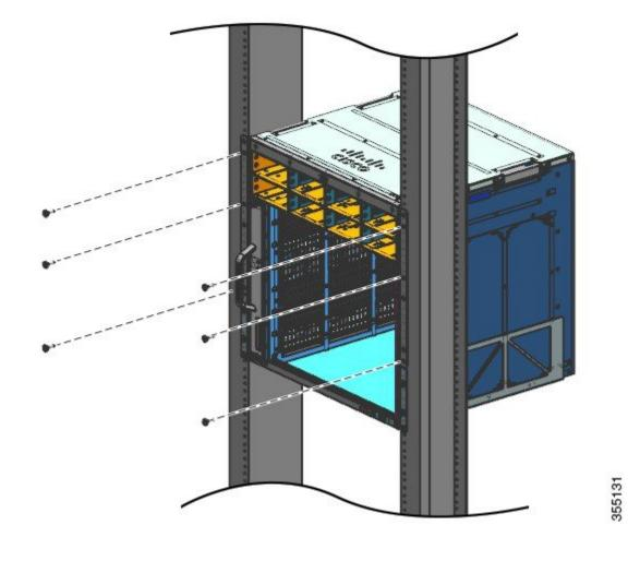
Figure 19: Securing the Chassis to the Rack Posts
