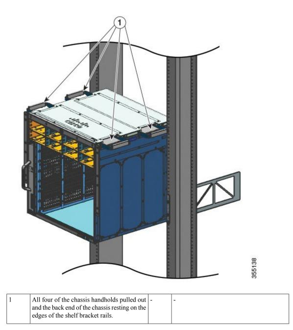
**Step 2** With a person standing at each side of the chassis, insert one hand into each handhold. Slowly lift the chassis. Avoid sudden twists or moves to prevent injury.
