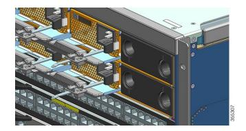
**Note** Power supply blank covers can be placed in any slot when fewer than eight power supplies are installed in a chassis.
