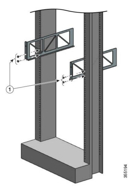
**Step 2** Using only one screw on each side, secure the L bracket to the rack rails.
