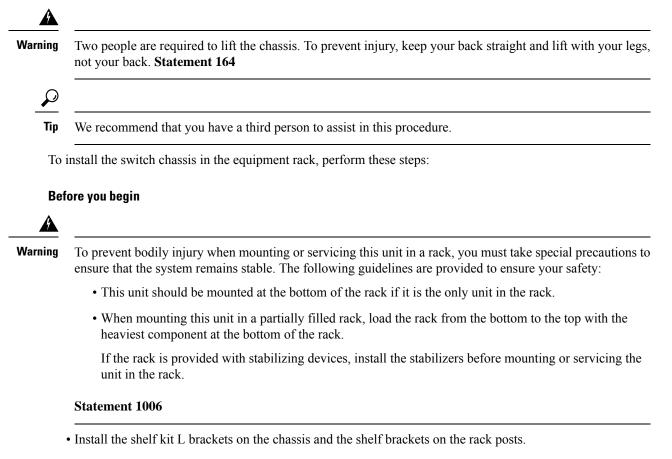
• Cable guide installation options have been described in a separate topic. If you are installing the cable guide, read this procedure and the cable guide installation procedure, before you start.
