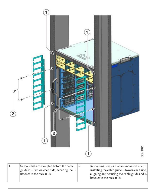
Cable guide installation without shelf brackets is complete.
