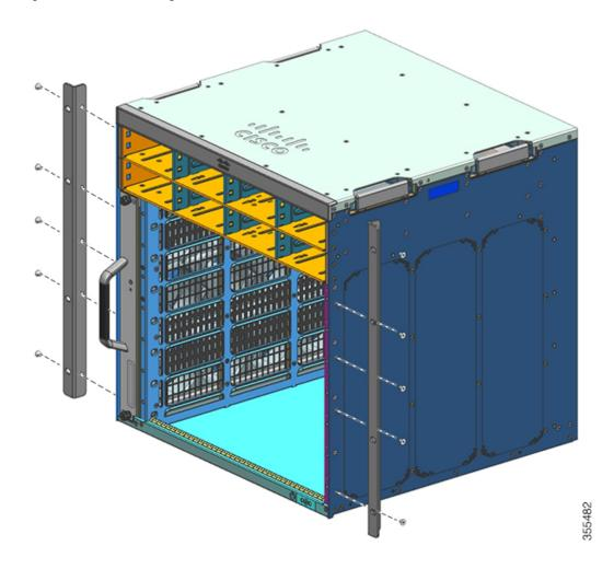
**Step 2** Install the rack ear brackets on the left and right sides of the chassis. These brackets connect the chassis to the rack.
