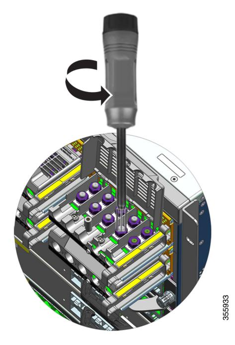
**Step 5** Attach the lug to the two posts, secure with the two nuts, and tighten with the torque driver. The fastening torque is between 2.0 and 2.8 Nm. Do not overtorque.
