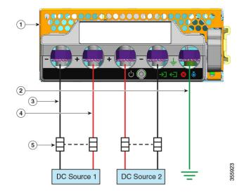
Figure 6: C9400-PWR-3200DC Installation Example: Separate DC Sources
