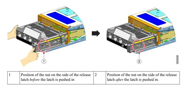
**Step 4** Grasp the terminal block with one hand. Place your other hand underneath as you slide the power supply module into the bay.
