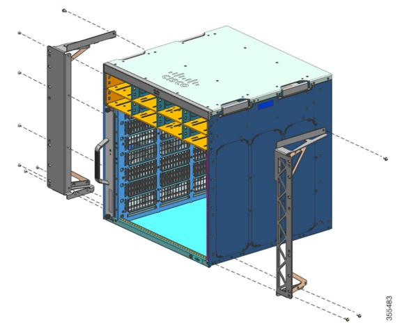
**Step 3** Install the filter brackets.
