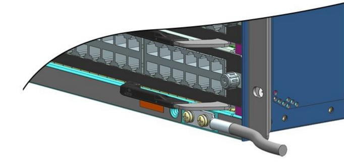
**Step 5** Prepare the other end of the grounding wire, and connect it to an appropriate grounding point in your site to ensure adequate earth ground for the switch.
