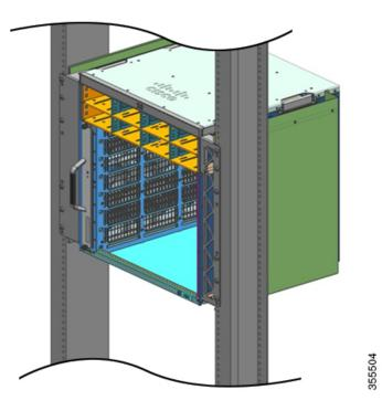
**Step 6** Slide the air filter into the air filter slot.
