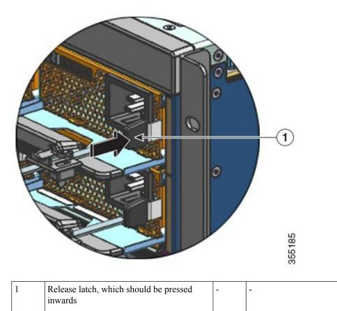
**Step 5** Grasp the power supply module with one hand; place your other hand underneath to support the bottom of the power supply. Slide it out of the bay completely.
