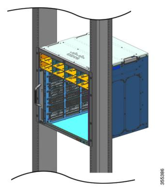
**Step 4** 4. Use a tape measure and level to ensure that the chassis is installed straight and level..
