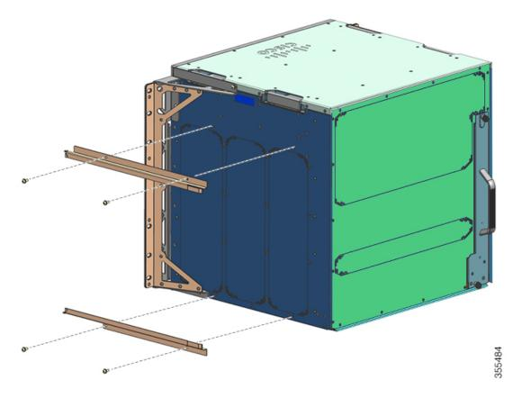
Step 4Install the Right and Left Wall covers.Figure 24: Install the Wall Covers
