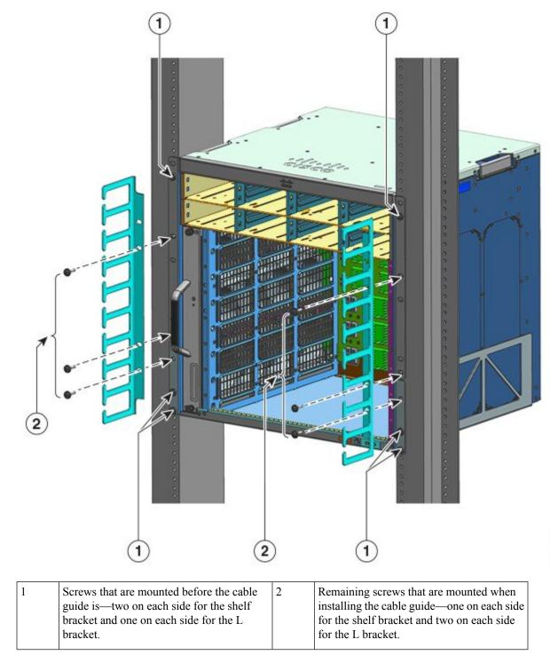
Cable guide installation with shelf brackets is complete.
