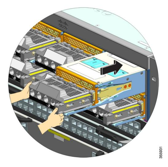
The following figure shows a power supply module that is fully installed in the bay:
