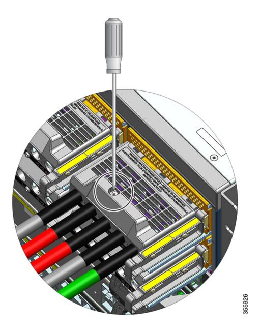
**Step 2** Using a nut driver, loosen the two nuts of one terminal slot at a time. After the lugs are removed, place the nuts back on the terminal posts and tighten.
