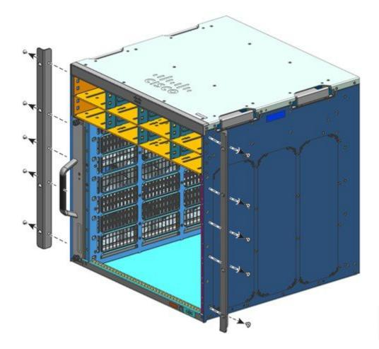
Figure 12: Removing L Brackets the Chassis is Shipped With
