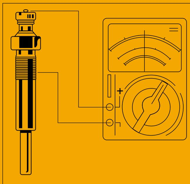
Resistance value ∞: The heating coil is broken
