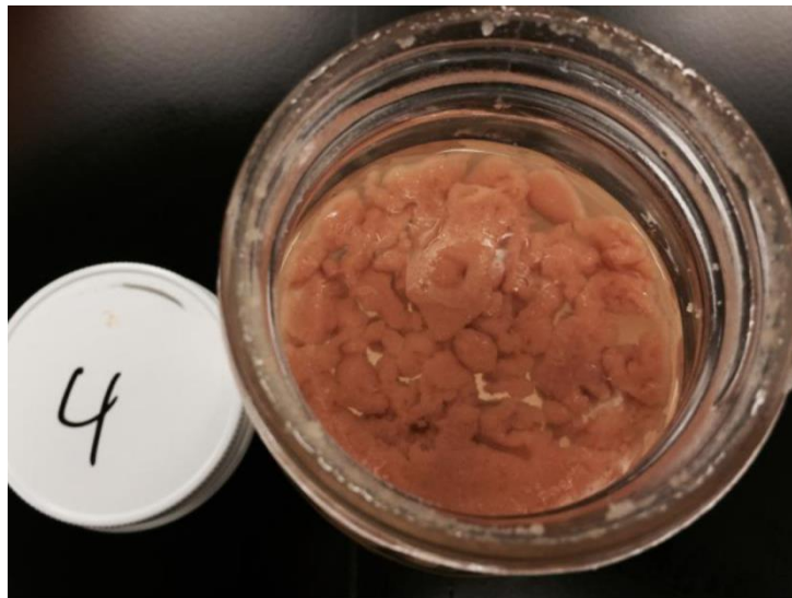
Fig 7: Saponification of Conventional Lubricants in Calcium Chloride Brine
