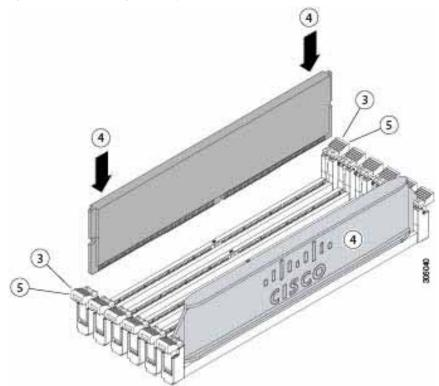
(4) Press evenly on both ends of the DIMM/PMEM until it clicks into place in its slot.
