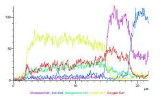
SEM image (left) and EDS line scan data (right) for Mn-Co coated T441 stainless steel sample exposed to an air atmosphere at 800 °C for 2000 hours. Image shows the good adhesion etween the 4  $\mu$ m chromia scale and T441 stainless steel.
