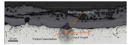
Use of pyramidal micro-indentation tests to characterize interfacial toughness for the interconnect scale.
