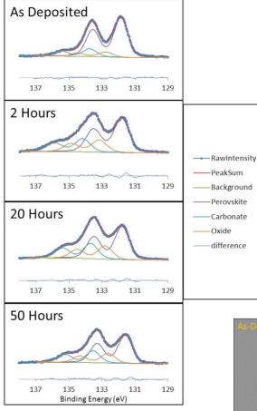
**Figure 1.** Curve fitted Sr 3D regions of the HAXPES spectra of LSCF 7328.
