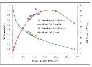
**Figure 2.** Polarization and power curves for DMFC model and experimental Data.
