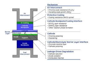
Schematic of a SOFC highlighting potential degradation mechanisms.
