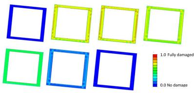
Progression of damage and healing of a viscous glass sealant during thermal-mechanical loading of an SOFC stack.
