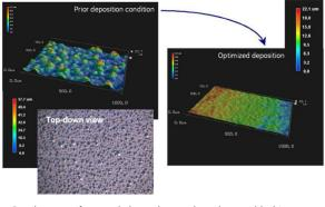
Development of a smooth thermal sprayed anode to enable thin thermal sprayed electrolytes.
