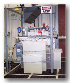
Photograph of pilot-scale electrodeposition cell for coating industrial scale SOFC interconnects.
