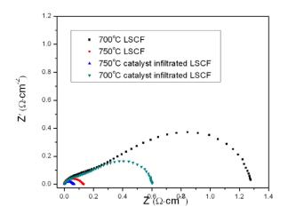
Figure 1. Nyquist plots of LSCF backbone and catalyst infiltrated LSCF cathode measured at 700 and 750 °C in air showing the decreased polarization resistance by infiltration.
