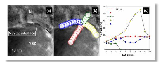
Figure 2: Yttrium migration along the Ni/YSZ interface in anode operated in syngas with 10 ppm PH<sub>3</sub> (a) nano structure of Ni/YSZ interface (a) location of sampling points: tetragonal YSZ domain (blue), cubic YSZ domain (yellow) (c) Profiles of Y/Zr ratio.
