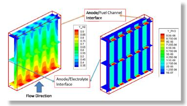
Figure 3: Results for mole fraction inside the anode from the degradation model after 2.5 hours of exposure to 10 ppm phosphine in 3% steam, 97% hydrogen fuel at about 850 °C.
