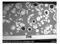
Figure 1: Scanning electron micrograph of a composite glass seal consisting of SEM-COM's crystallization-resistant multi-component silicate glass, SCN-1, and frangible hollow calcia-stabilized zirconia particles. The fracture of the hollow spheres under the application of a compressive load gives the composite glass seal the ability of filling uneven spaces, for example, when sealing surfaces that are not parallel or flat.
