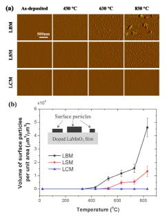
**Figure 1.** (a) AFM amplitude images of the Ba-, Sr- and Cadoped LaMnO<sub>3</sub> thin film surfaces as a function of annealing temperature. Each column represents the surface morphology after annealing in air for 1 hour at the temperatures stated on the top. Each row represents the surface morphology of LBM, LSM, and LCM. (b) The volume per unit area of the surface particles, calculated from the AFM images, as a function of annealing temperature for LCM, LSM and LBM.
