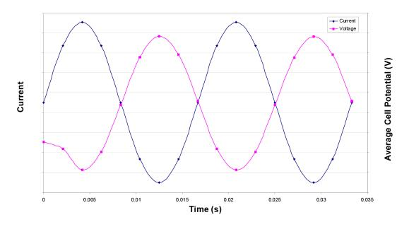
Figure 2. Voltage response of cells to sinusoidal input current signal.
