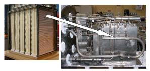
Assembly of 5 LGFCS SOFC strips into a block configuration (left) having a nominal power output of 19 kW and inclusion within the pressurized test rig (right) that incorporates product-level system technology and operates at conditions representative of future commercial systems.
