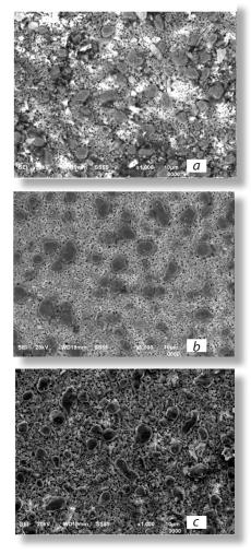
Figure 1: Microstructure images of anode aged in dry  $H_2$  with 10 ppm PH<sub>3</sub> obtained using Environmental Scanning Electron Microscope (ESEM): (a) Initial at 25 °C (b) after 6 hours at 800 °C (c) final at 25 °C
