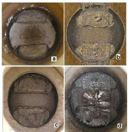
Figure 4: Post-mortem PH<sub>3</sub> poisoned cell anodes (2 cm diameter). (a) syngas at 750 °C, (b) syngas at 850 °C, (c) dry H<sub>2</sub> fuel at 800 °C and (d) dry H<sub>2</sub> fuel without load at 800 °C.
