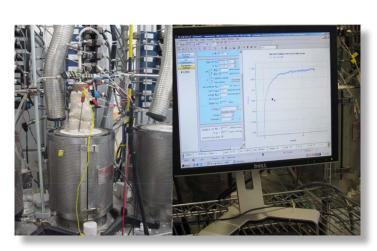
*Electrochemical test facility capable of testing under "real world" air exposure conditions.*
