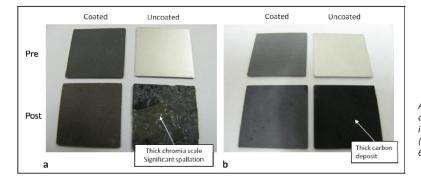
Appearance of coated and uncoated 304 austenitic stainless steel after (a) 500 hours in an oxidizing atmosphere at 900 °C; and (b) 24 hours in a coking atmosphere at 600 °C.
