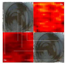
**Figure 1:** Comparison of the Co (bottom left) and Fe (top right) mapping with an actual picture (top left, bottom right) of the sample surface of the positive side of sample (with GDC interlayer, 500 mV applied bias during heat treatment). White lines as guide to the eye point out prominent structures in the picture and their counterpart in the map.
