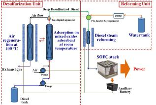
The Conceptual Design for Diesel Fuel Processor using the Deep Desulfurization Adsorbent and the Low-cost Fe-Ni Bimetallic Steam Reforming Catalyst Developed in this Project for SOFC.
