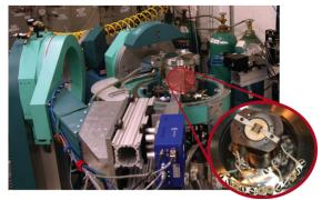
The environmental chamber mounted on the 12ID-D diffractometer at the Advanced Photon Source. The inset shows the sample that is within the beryllium windowed chamber.
