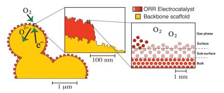
A schematic drawing of a heterostructured SOFC cathode depicting the variation in chemistry and structure going from the micro- to the nanoscale. At the nanometer length scale, the solid-gas interface is very different from the bulk in terms of structure, composition, and electronic structure. The backbone scaffold conducts oxygen ions and electrons to and from the electrolyte and external circuit respectively, and the electrocatalyst facilitates the surface reaction.
