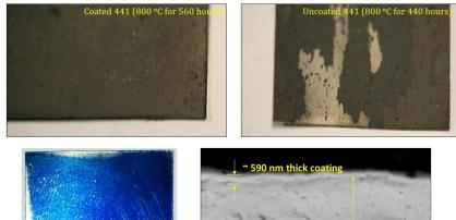
Images of ~1"x1" coupons of  $(Mn,Co)_{3}O_{4}$  coated and uncoated 441 SS following oxidation in ambient air at 800 °C. The coated scale remains adhered while large portions of the uncoated scale have spalled.
