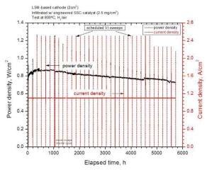
Long-term degradation test of a button cell infiltrated with an engineered SSC (strontium-doped samarium cobaltite) catalyst via the single-step VPIT process.
