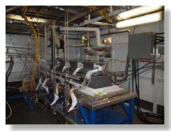
Test room with SOFC Breadboard for Four Stack Assembly.
