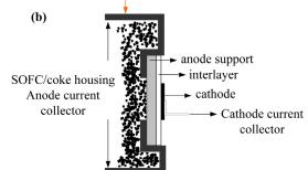
(a) Schematic of the coal injection and fly ash withdraw system(b) Side view of the coal SOFC compartment
