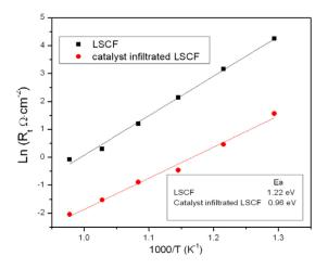
Figure 2. Polarization resistance as a function of inverse temperature. The performance of a noninfiltrated cell is provided for comparison. The activation energy of LSCF cathode is reduced by infiltration.
