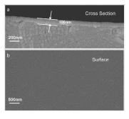
Figure 2. (a) A cross-sectional and (b) a surface view of the LSCF thin film deposited on a gadolinia-doped ceria substrate by a radio frequency sputtering technique after annealing at 800°C for 1 hour.
