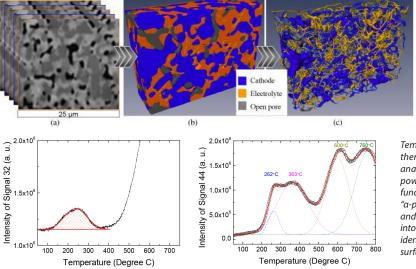
Schematic showing the transition from scanning electron image stack (a), which is used to generate a three-dimensional (3-D) reconstruction (b), which is then reduced to a mass centroid 3-D skeleton (c).
