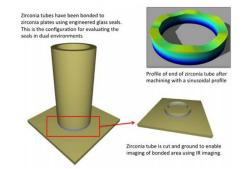
Figure 2. Experimental procedure used to demonstrate the ability of engineered glass seals to seal surfaces that are not flat and/or parallel. The inset shows the end of the zirconia tube that had been machined with a sinusoidal profile with an amplitude of 75 µm. The integrity of the joint was examined by infrared imaging and its hermeticity was evaluated using a dual environmental test set-up.
