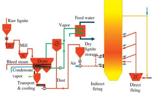
Figure 4-1 External Pre-drying System based on Fluidized Bed Drying Technology for Lignite Firing
