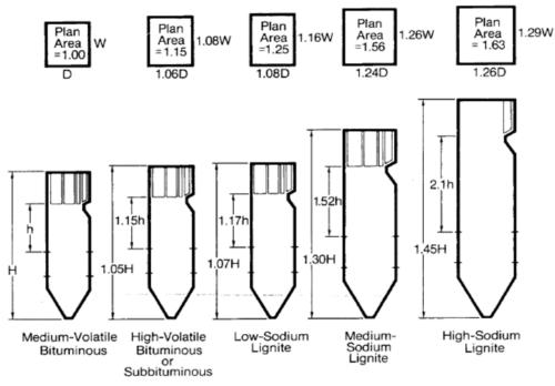
Figure 3-1 Impacts of Coal Properties on Boiler Sizing
