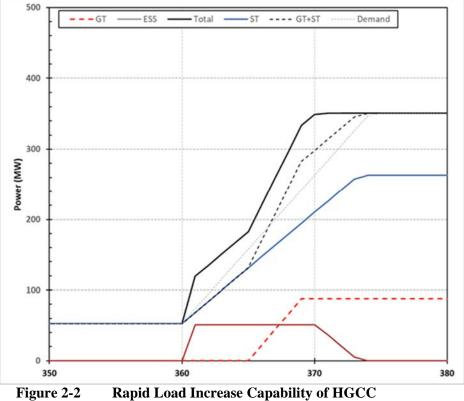
Figure 2-2 Rapid Load Increase Capability of HGCC
