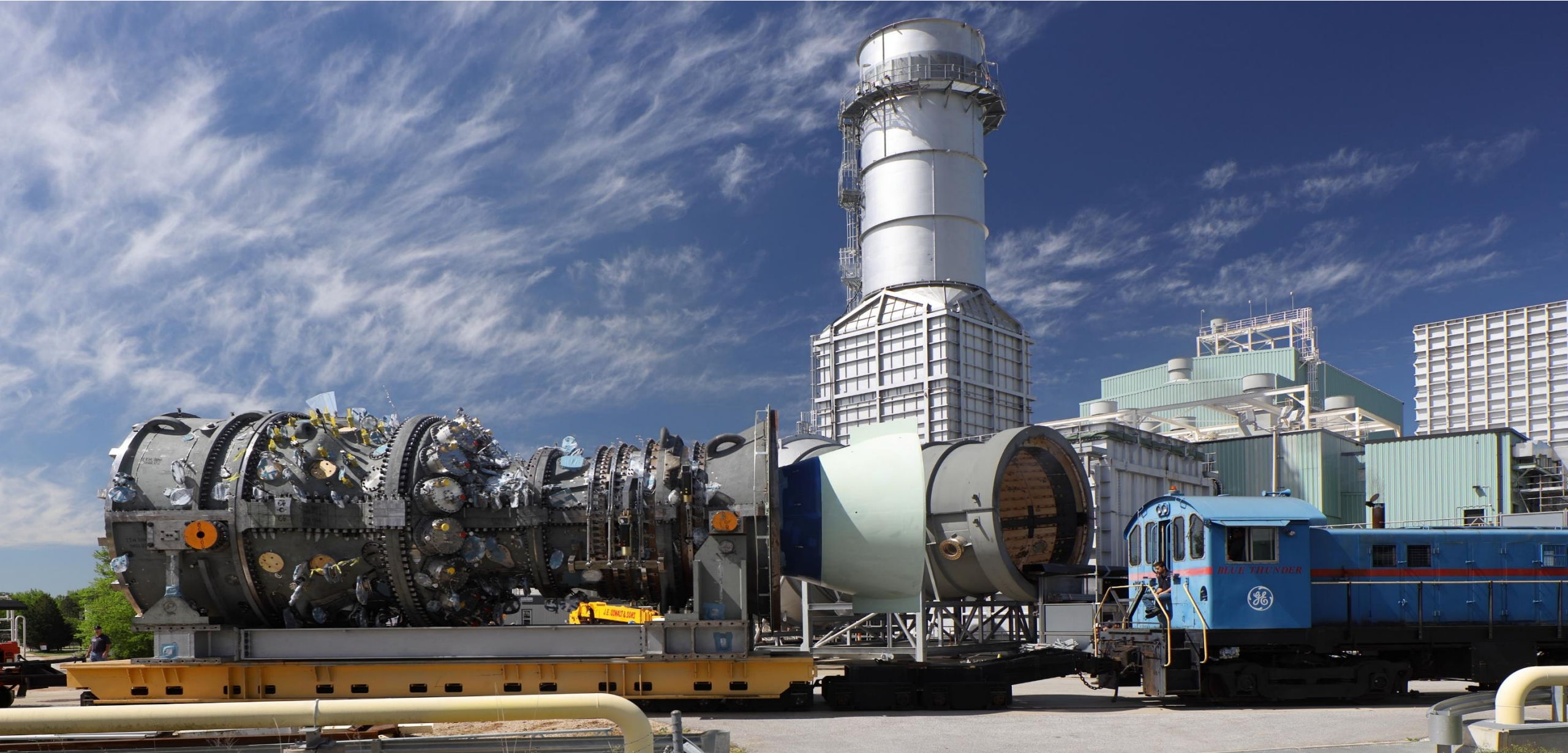
First Production 9HA.02 for Full-Speed, Full-Load Testing & Validation at GE Greenville
