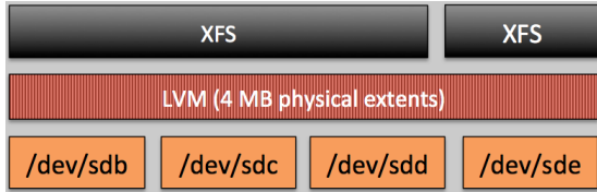
Fig. 3. Schematic of the different layers of the DataWarp software. The Burst Buffer node is logically 4 SSD block devices, which are aggregated by LVM. When a Burst Buffer allocation is requested by the user, an XFS filesystem is created by the DataWarp software on that allocation. In this example, two different allocations coexist on the same Burst Buffer node
