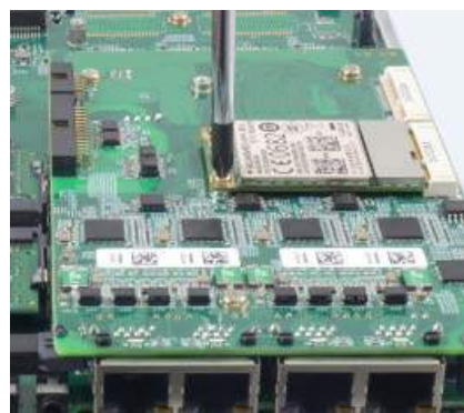
Secured with M2.5 P-head screw
