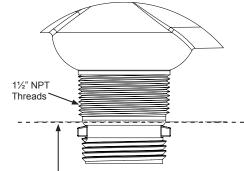
Quick Connect Nut Threads can be cut off to allow access to 11/2" NPT Threads. Deburr and clean edge after cutting. **NOTE:** Teflon tape is required when using the 1½" NPT Threads.
