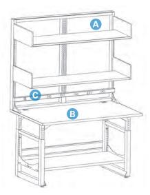
A Strong, durable, modular steel TechOrganizer allows for a myriad of desktop and overhead storage accessories and options. Helps to keep worksurfaces clear and contributes to proper 'lean' lab management principles.
