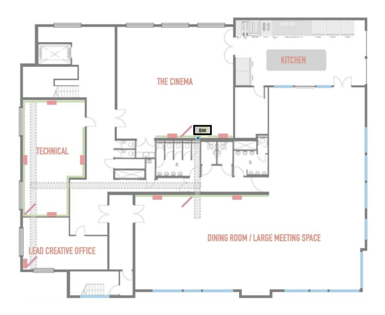
Despite the size of the upstairs, only 18 network ports have been positioned on the floor plan. The switch will be connected back via a fibre cable to the core switch in the server room. The ceiling already has the cable tray installed so the challenge of running the cable back to the single switch is relatively simple to overcome.
