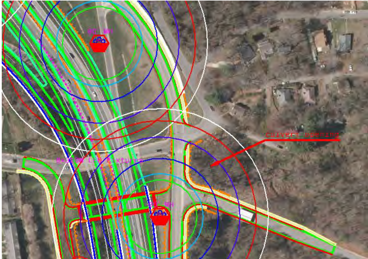
Figure 22: Original lighting layout at Hill Street culvert inlet.
