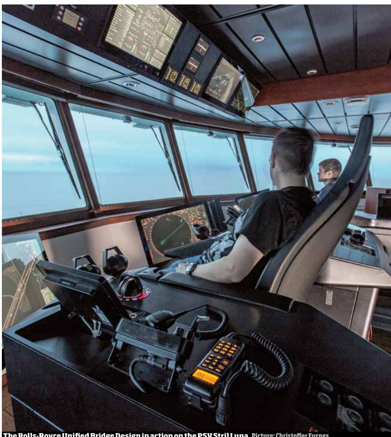
The Rolls-Royce Unified Bridge Design in action on the PSV Stril Luna Picture: Christoffer Furnes
