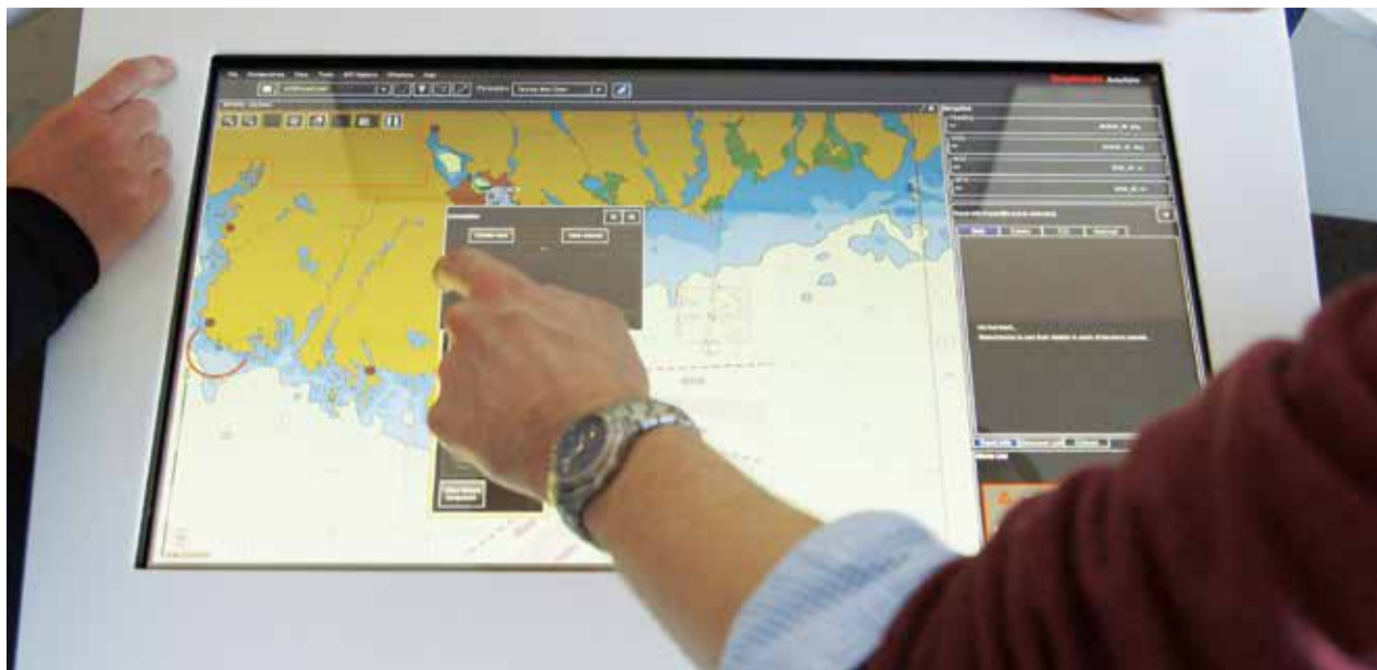
The Shared Display enables seafarers to annotate charts and leave messages for colleagues
