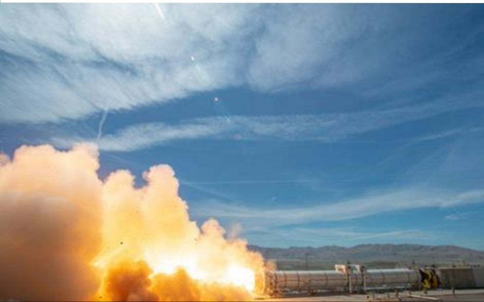
Successful Solid Rocket Motor Hotfire
