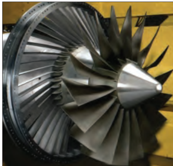
Swept and leaned strators—technology for noise reduction.
