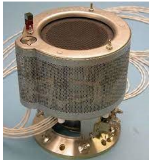
Figure 4.31: T5 gridded-ion thruster for GOCE mission. Credit: QinetiQ.
