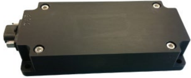
Figure 5.4: NSS Magnetometer. Credit: NewSpace Systems.
