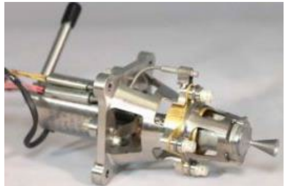
Figure 4.6: GR1 thruster. Credit: Aerojet.
