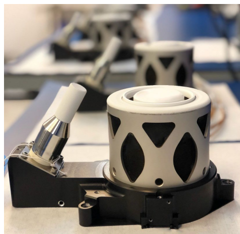
Figure 4.42: BHT-350 Flight Units. Credit: Busek Co.
