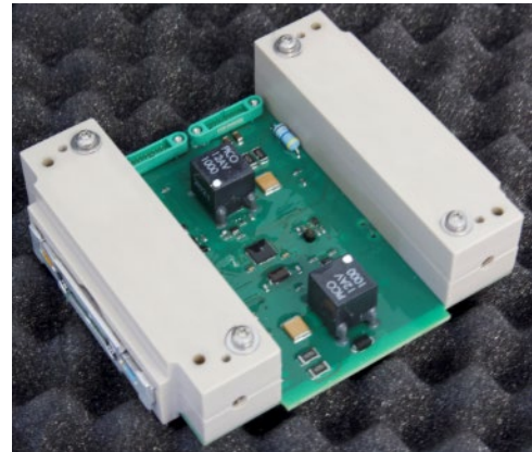
Figure 4.50: Plasma Brake Module (PBM) demo unit. Credit: Aurora Propulsion Technologies.
