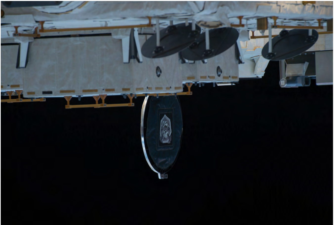
View of CATS on the Japanese Experiment Module Exposed Facility (ISS049E006036).
