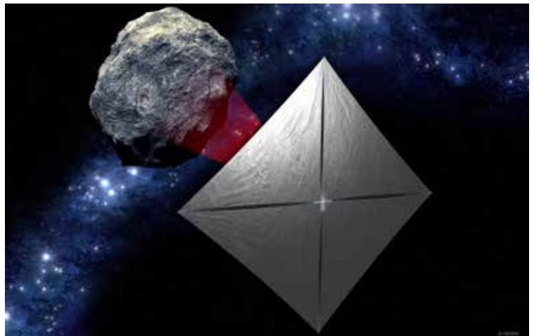
Artist concept of Artemis I secondary payload, NEA Scout, with its deployed solar sail on its way to an asteroid.
