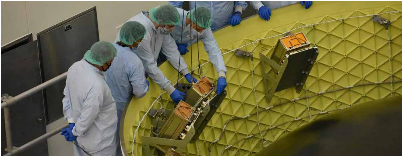
The Jacobs team at NASA Kennedy installing the last of 10 CubeSats in the SLS rocket's Orion stage adapter. BioSentinel, the final CubeSat to be loaded, will study how radiation affects living organisms in deep space.
