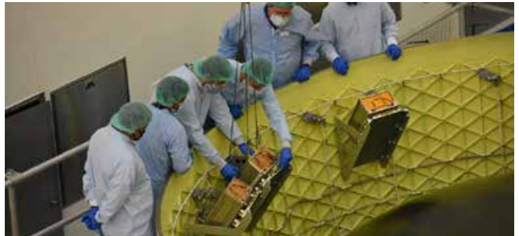
The Artemis I Orion stage adapter with mounting brackets for secondary payloads.
