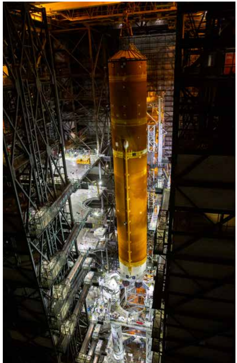
The SLS core stage, the tallest rocket stage NASA has ever built, is lowered between the Artemis I boosters in the Vehicle Assembly Building.
