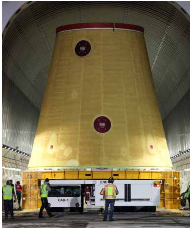
The launch vehicle stage adapter adapter partially encloses the ICPS and contains the pyrotechnic system to separate itself and the core stage from the ICPS and Orion.
