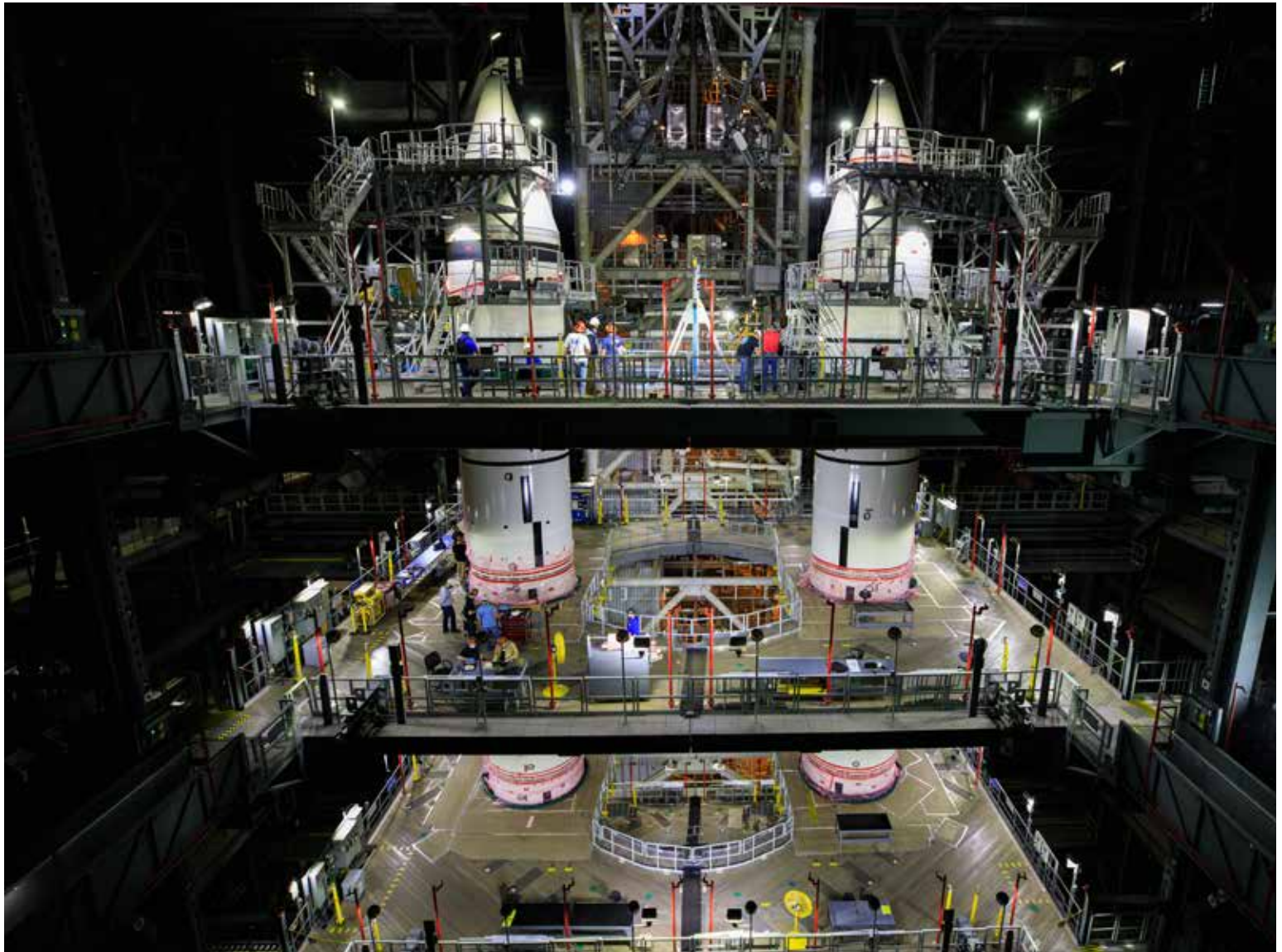
The five-segment SLS solid rocket boosters generate 7.2 million lbs. (32,027 kN) of thrust – more than 75 percent of the vehicle's total thrust for the first two minutes of flight.
