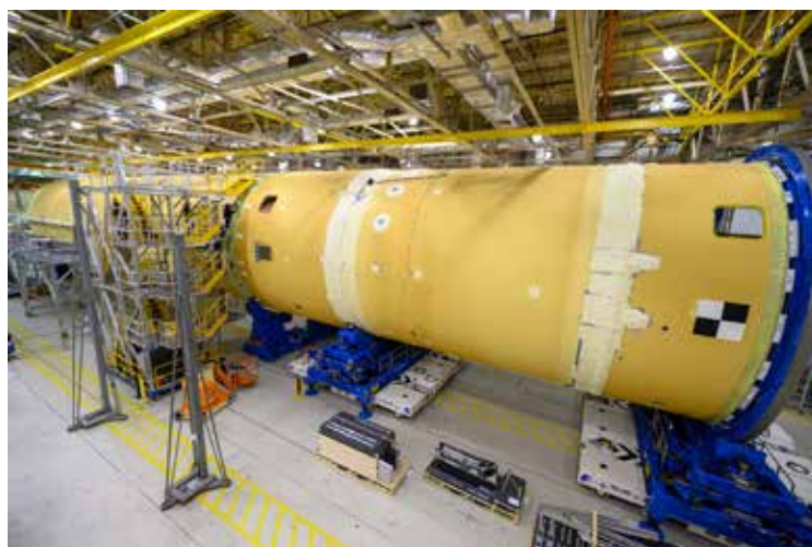
Connecting feedlines and other external components to the fully assembled Artemis I core stage at Michoud.
