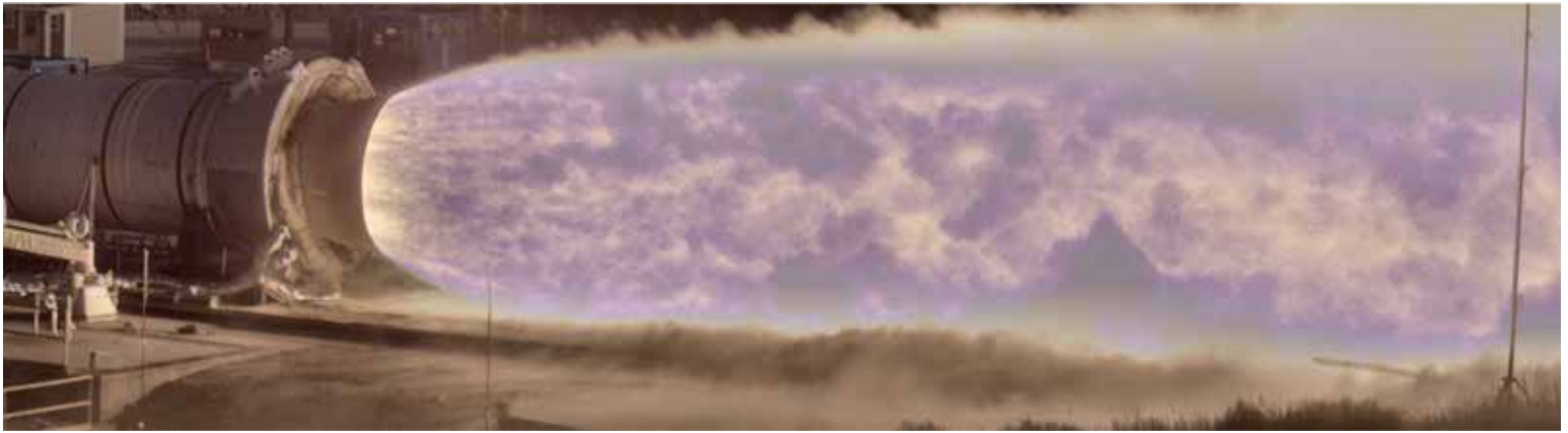
Boosters lead contractor Northrop Grumman and NASA hot-fired several full-scale solid rocket motors to help qualify them for the SLS Program.
