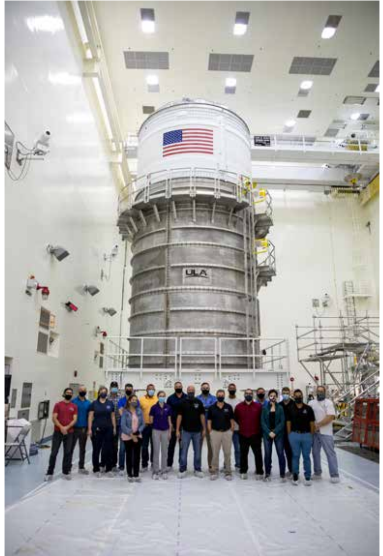
ULA supplies the ICPS, which is based on the Delta Cryogenic Second Stage, for the SLS Block 1 rocket.
