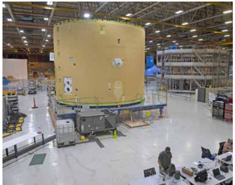
The SLS Artemis I intertank at Michoud, prior to integration between the propellant tanks, has forward attach points for the two solid rocket boosters.
