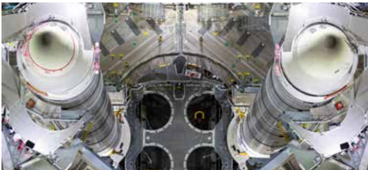
Artemis I five-segment solid rocket boosters stacked on the mobile launcher.
