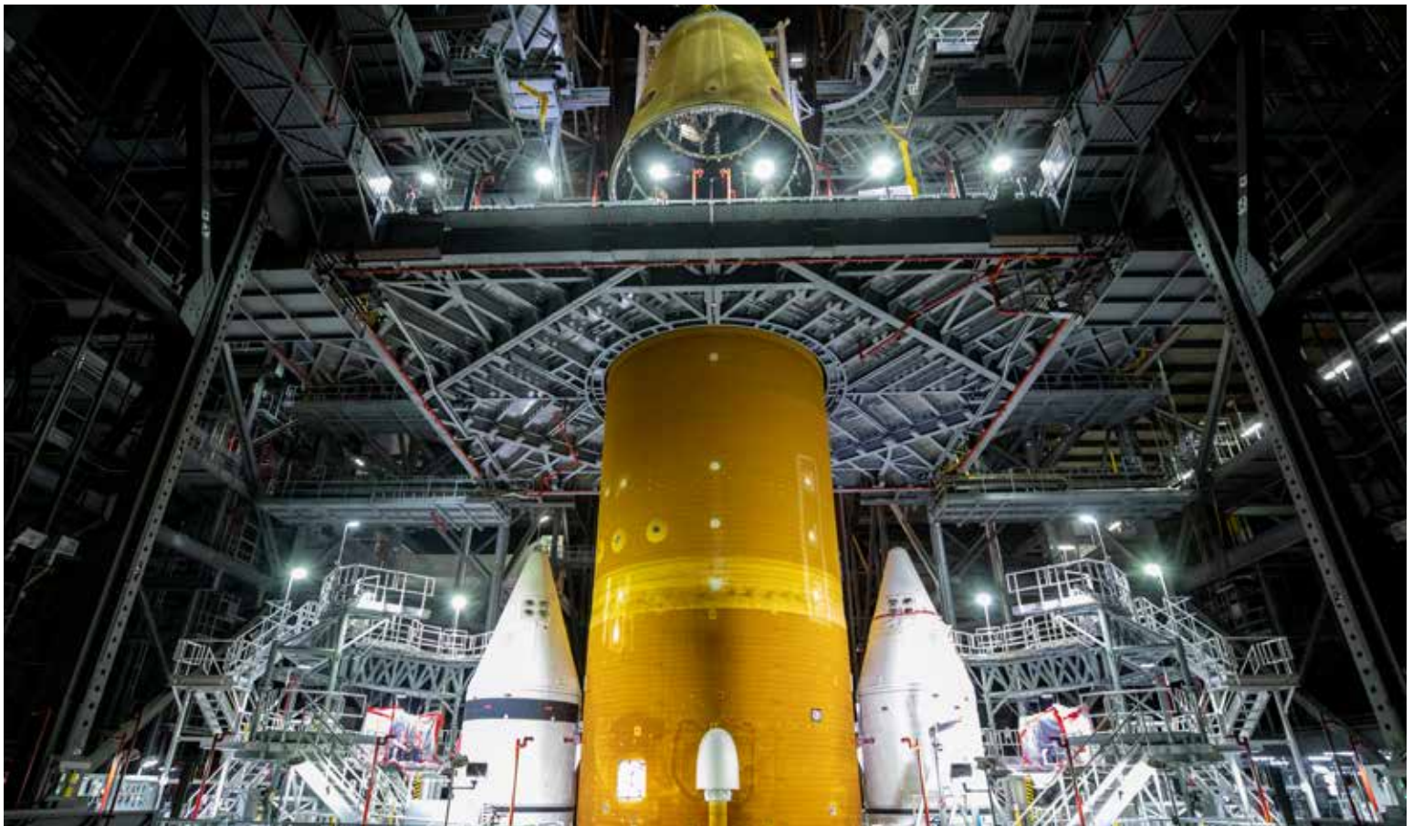
The SLS gets its signature orange color when its spray-on foam insulation darkens with exposure to sunlight. The core stage below the work platform was exposed to months of sunlight during Green Run testing at Stennis, while the launch vehicle stage adapter being lowered into place above the platform has been stored indoors since its completion.
