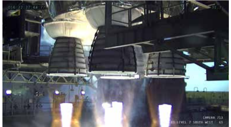
The Artemis I RS-25 liquid fuel engines operated successfully as part of the core stage Green Run hot fire test at Stennis in early 2021.
