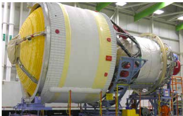
The ICPS is a single-engine liquid hydrogen/liquid oxygen stage based on the Delta Cryogenic Second Stage from ULA that produces 24,700 lbs. (110 kN) of thrust and performs the TLI burn to send Orion toward the Moon.
