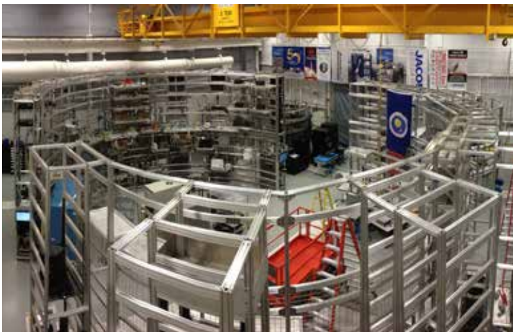
The Systems Integration Lab/Systems Integration Test Facility at Marshall is a full-scale mockup of flight-like avionics systems for the solid rocket boosters and core stage where engineers can test hardware and software integration prior to manufacture and flight.
