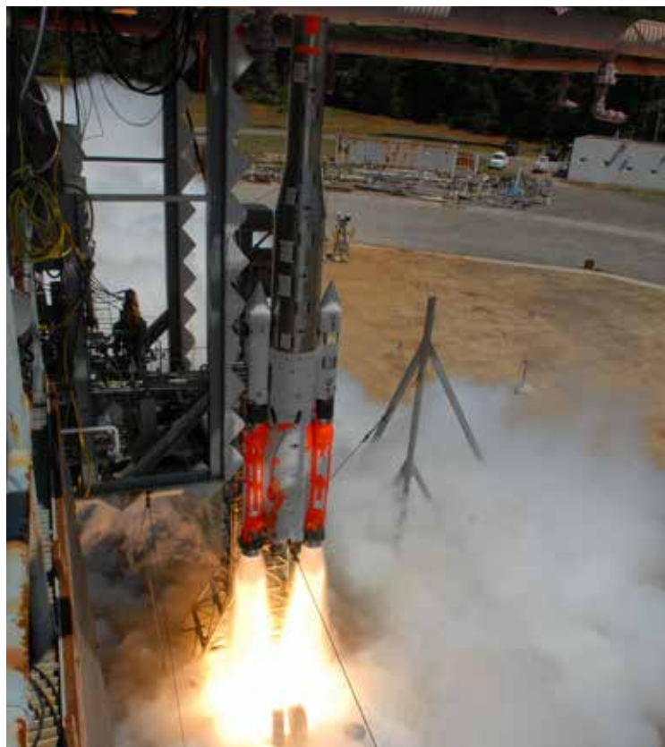
A five-percent scale model of SLS undergoes acoustic testing in 2014 at Marshall.
