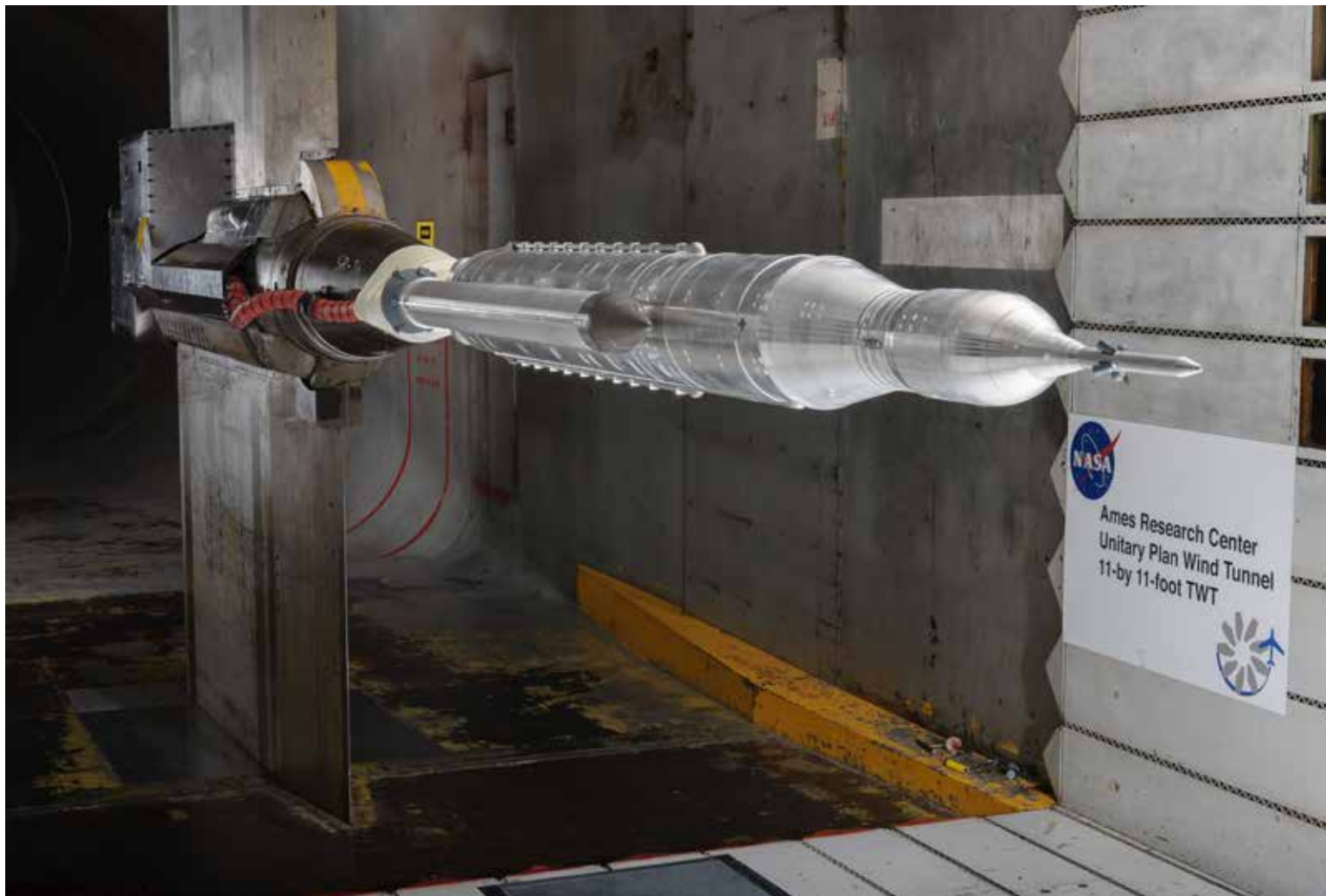
A scale model of SLS was tested in an 11-by 11-ft. (3.4-by 3.4-m) Transonic Wind Tunnel at Ames. Data from the wind tunnel tests at Ames and Langley was used to improve the design and stability of SLS.
