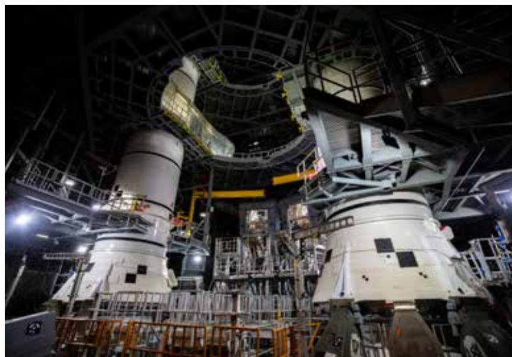
The solid rocket boosters' aft assembly includes the aft skirts with thrust vector control system inside that helps steer SLS during ascent. The entire weight of the SLS vehicle goes through the aft skirt structures.
