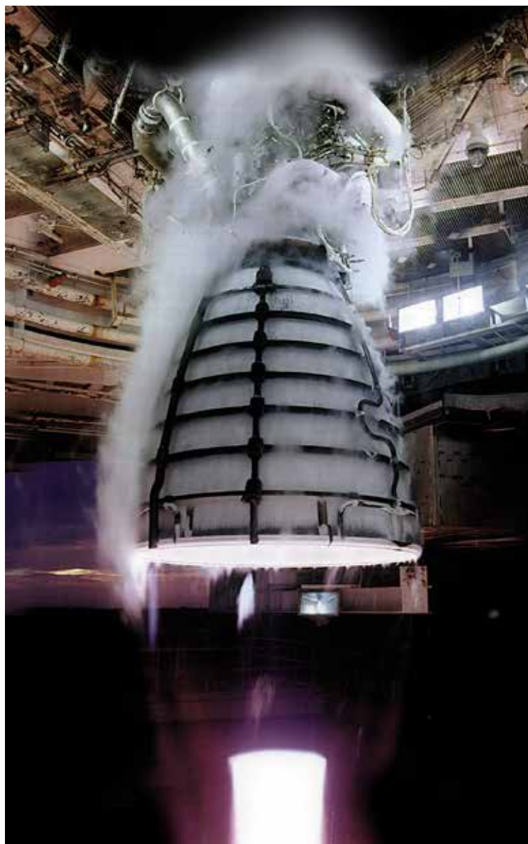
The RS-25s have been upgraded with new controllers that were hot-fire tested prior to the Artemis I flight.
