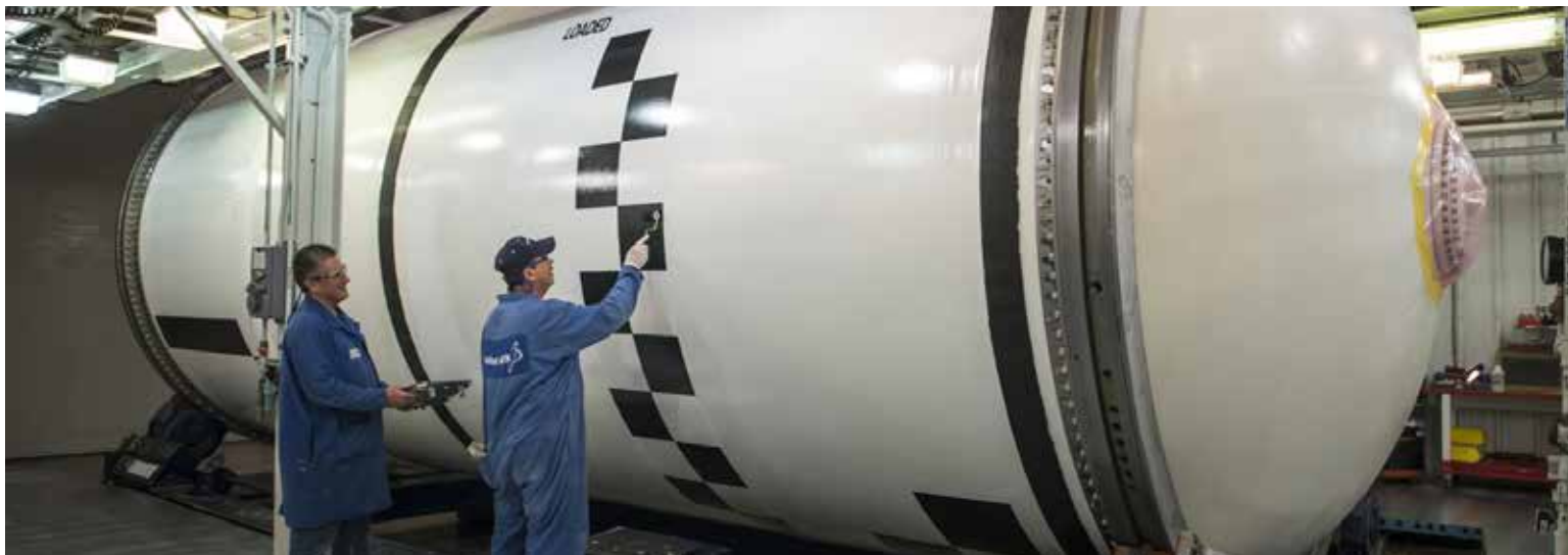
Technicians with lead solid rocket boosters contractor Northrop Grumman paint photogrammetric markings on one segment of an SLS solid rocket motor. The black-and-white targets painted on each element of the vehicle provide targets for cameras, which then use those positions compared with fixed positions on the ground and on the mobile launcher to precisely locate SLS in space.
