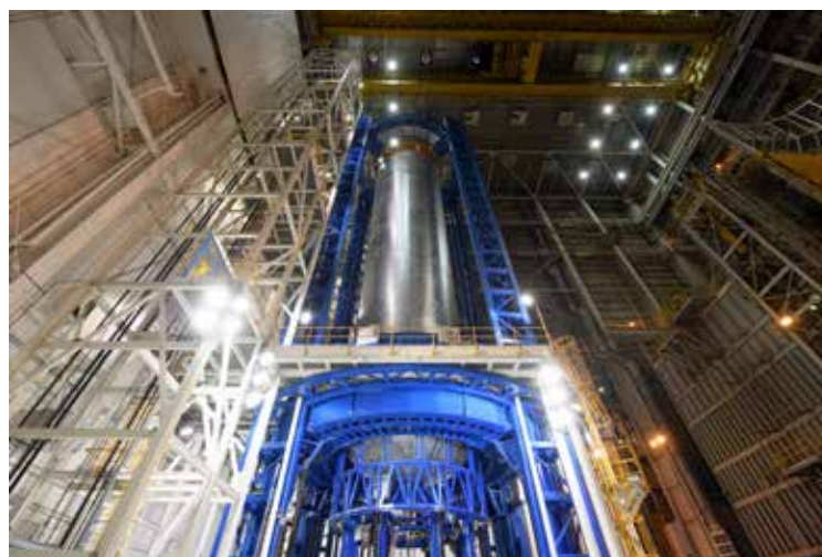
The Vertical Assembly Center at Michoud is one of the world's largest welding tools and is used to execute vertical friction-stir welds of the SLS core stage liquid hydrogen tank.
