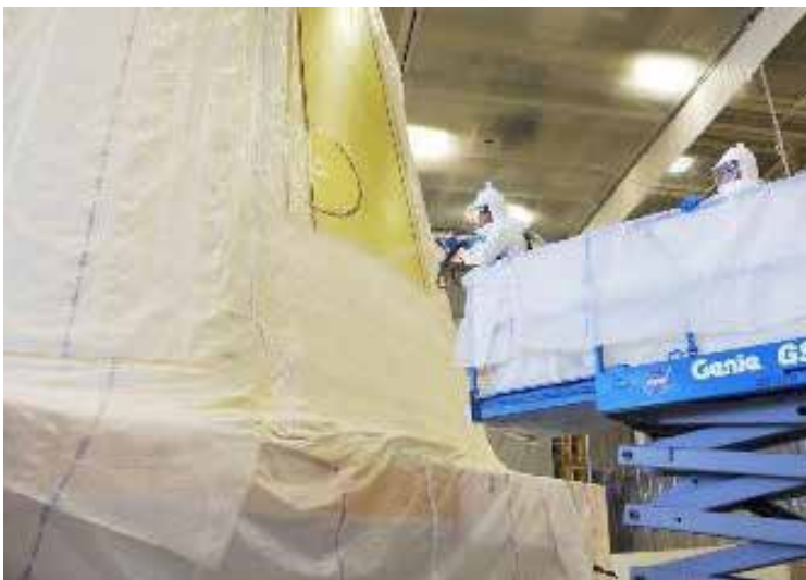
Teledyne Brown Engineering manufactures the launch vehicle stage adapter at Marshall, where technicians manually apply spray-on insulation, which turns orange in sunlight.
