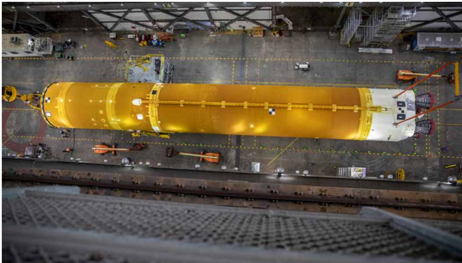
The 212-ft. (64.6 m) core stage for Artemis I in the transfer aisle of the Vehicle Assembly Building in preparation for lifting and integration on the mobile launcher. Manufactured by Boeing at Michoud, the stage houses the four RS-25 engines, propellant tanks, and flight computers. Too large to ship over land, NASA's barge Pegasus transported the Artemis I core stage to Stennis for a 'Green Run' test campaign and then to Kennedy for integration with the rest of the vehicle.
