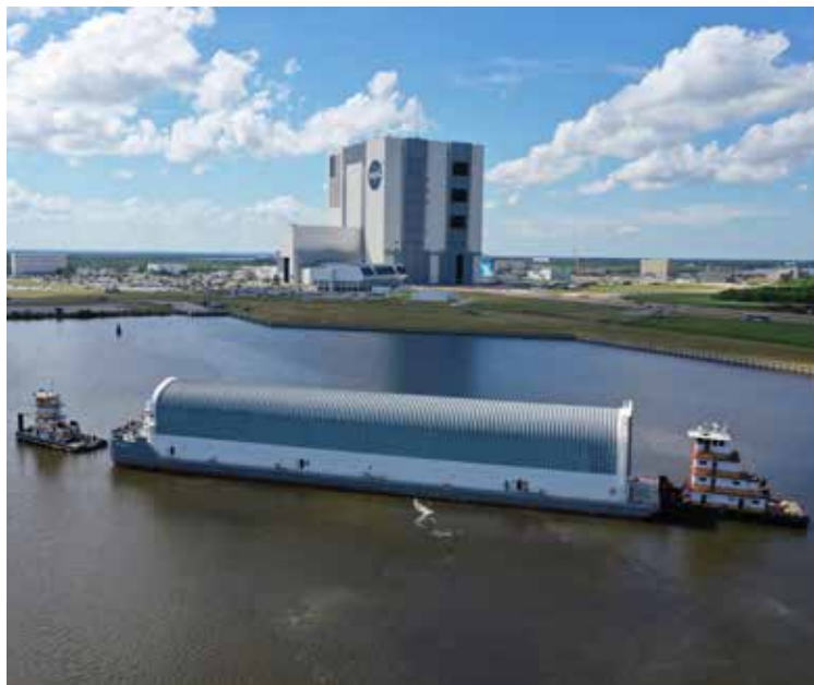
NASA's barge Pegasus , used to transport external tanks during the Space Shuttle Program, was lengthened and strengthened to transport the SLS core stage. A 115-ft. (35 m) section of the barge was removed and replaced with a specially reinforced 165-ft. (50 m) section to increase the weight Pegasus can carry. The length of the barged increased from 260 ft. (79 m) to 310 ft. (94 m).
