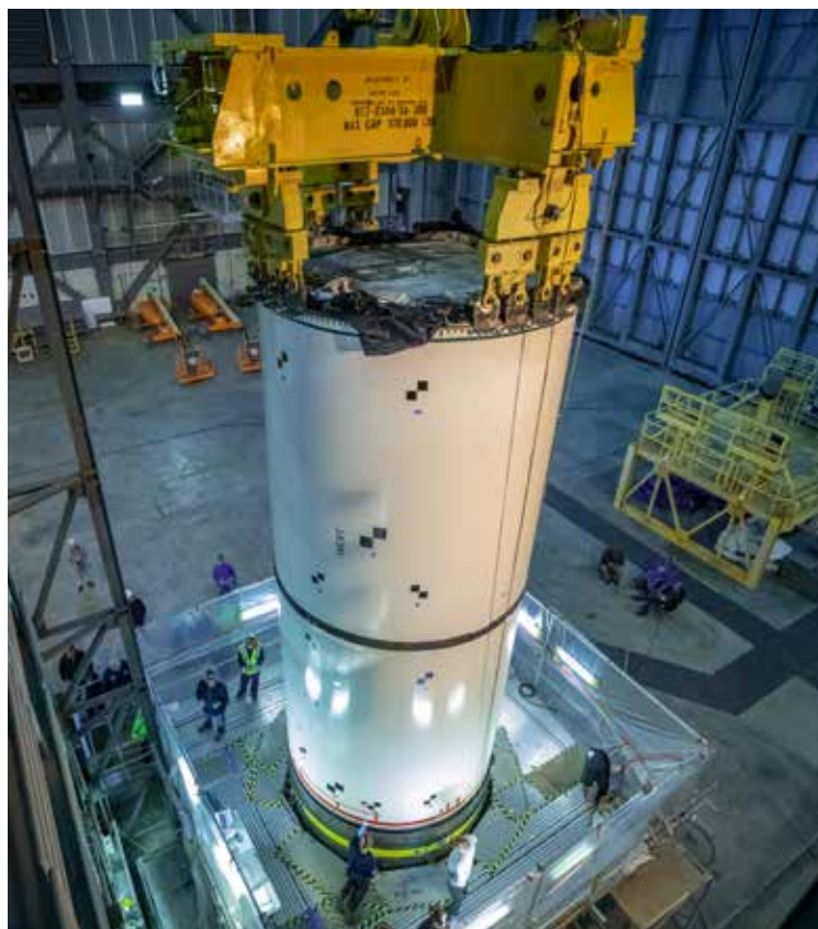
EGS and Jacobs technicians worked with inert booster motor segments as pathfinders in Kennedy's Rotation, Processing, and Surge Facility (RPSF) and Vehicle Assembly Building before assembling the Artemis I booster motor segments.
