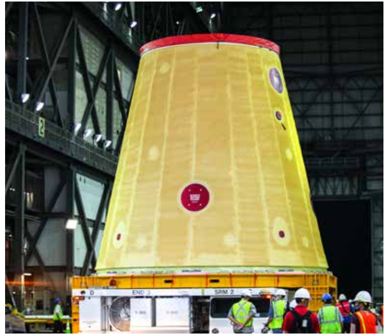
The Artemis I launch vehicle stage adapter arrives at the Vehicle Assembly Building for stacking on the Artemis I launch vehicle.
