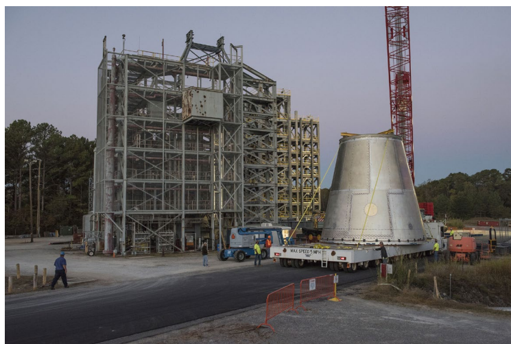
The launch vehicle stage adapter structural test article for the Integrated Structural Test was manufactured and tested at Marshall.
