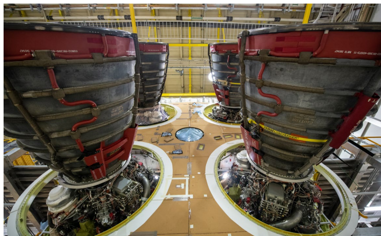
The Artemis I RS-25 engines installed in the core stage during assembly at NASA's Michoud Assembly Facility in New Orleans.
