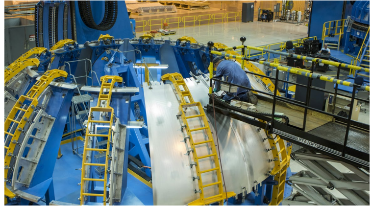
The gore weld tool at Michoud is used to weld domes for the SLS core stage propellant tanks.
