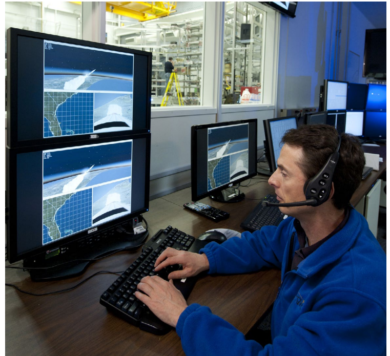
Marshall's Systems Integration Lab has the capabilities to allow the software team to fly thousands of virtual launches in a simulated environment that included wind, weather, and Earth's rotation.
