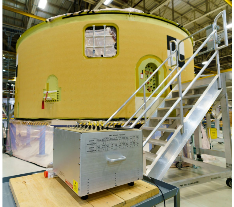
The core stage forward skirt contains the flight computers for the Block 1 SLS rocket.
