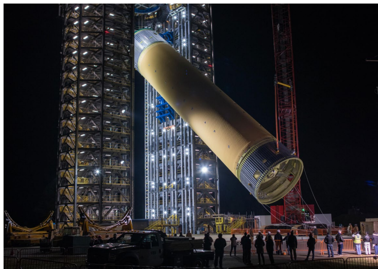
Technicians installed the liquid hydrogen tank structural test article in its test stand at Marshall at night when winds were minimal.
