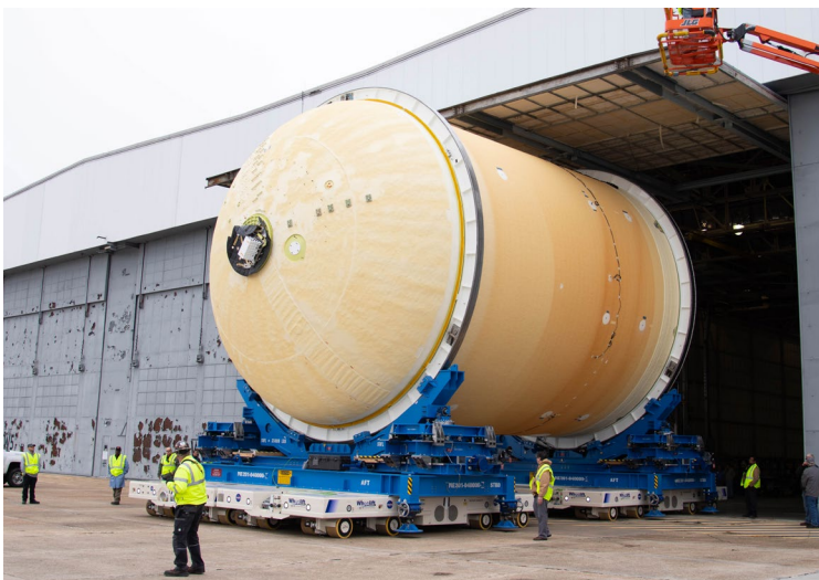
The liquid oxygen tank being manufactured for the Artemis I flight at Michoud.
