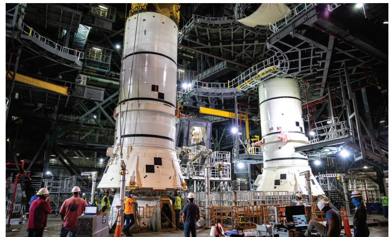
Artemis I booster aft assemblies ready for stacking in Kennedy Vehicle Assembly Building.
