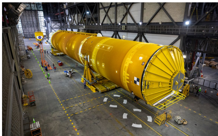
The Artemis I core stage waits in the Vehicle Assembly Building transfer aisle before stacking on the mobile launcher.
