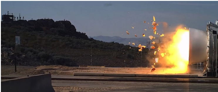
Close-up view of the throat plug break up and expulsion from the nozzle during ignition of the Qualification Motor 2 full-scale test firing in Utah.
