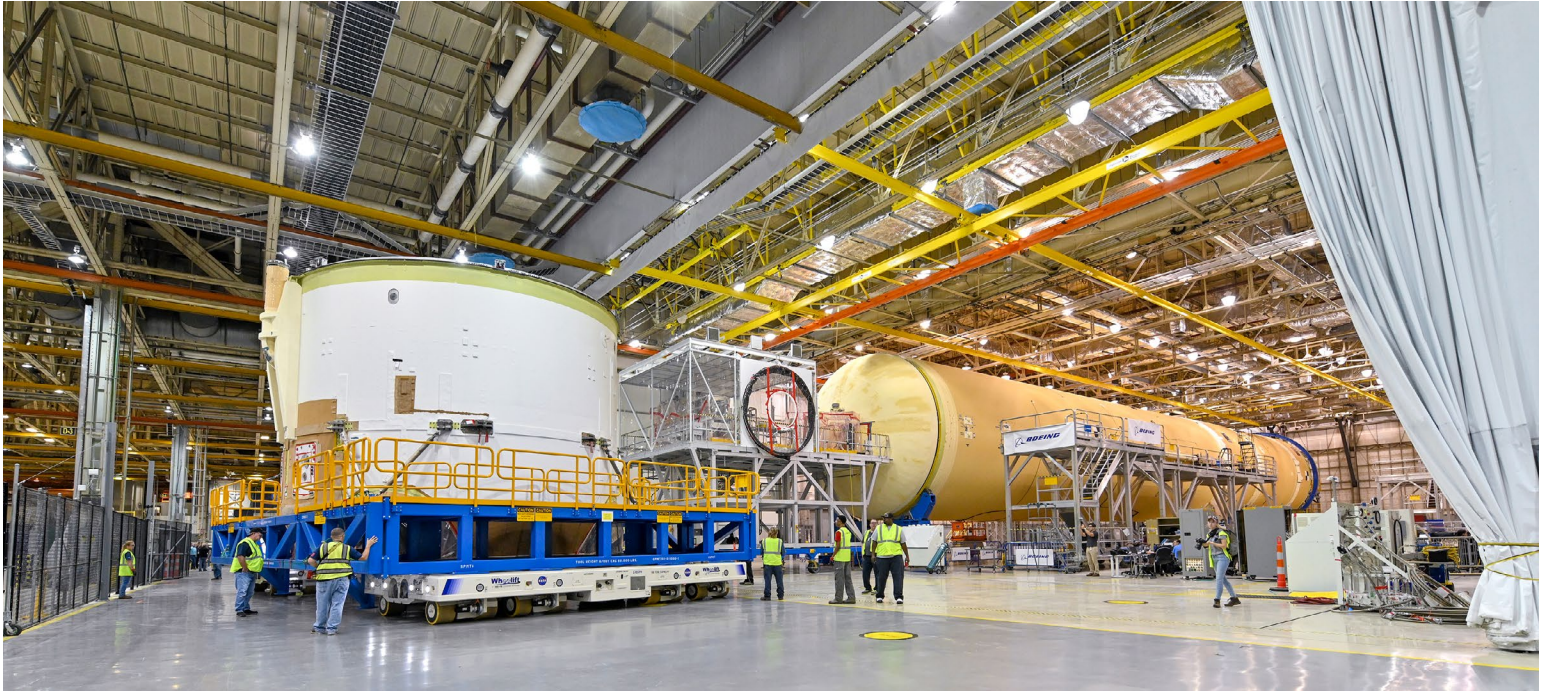
The SLS Artemis I engine section, left, and liquid hydrogen tank, right, at Michoud prior to integration.
