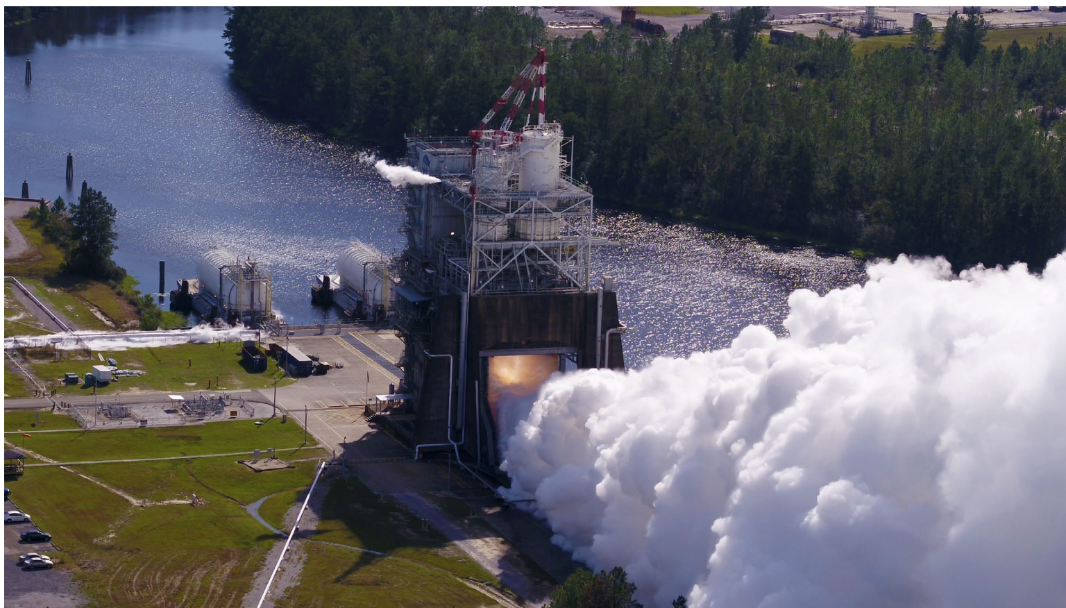
RS-25 hot fire testing at NASA's Stennis Space Center in Bay St. Louis, Mississippi, helped qualify engines to extreme SLS environments.
