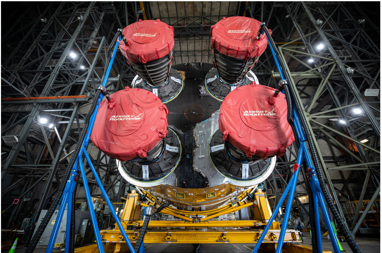
Industry partner Aerojet Rocketdyne, headquartered in Sacramento, California, supplies RS-25 engines for the SLS core stage and RL10 engines for the ICPS.
