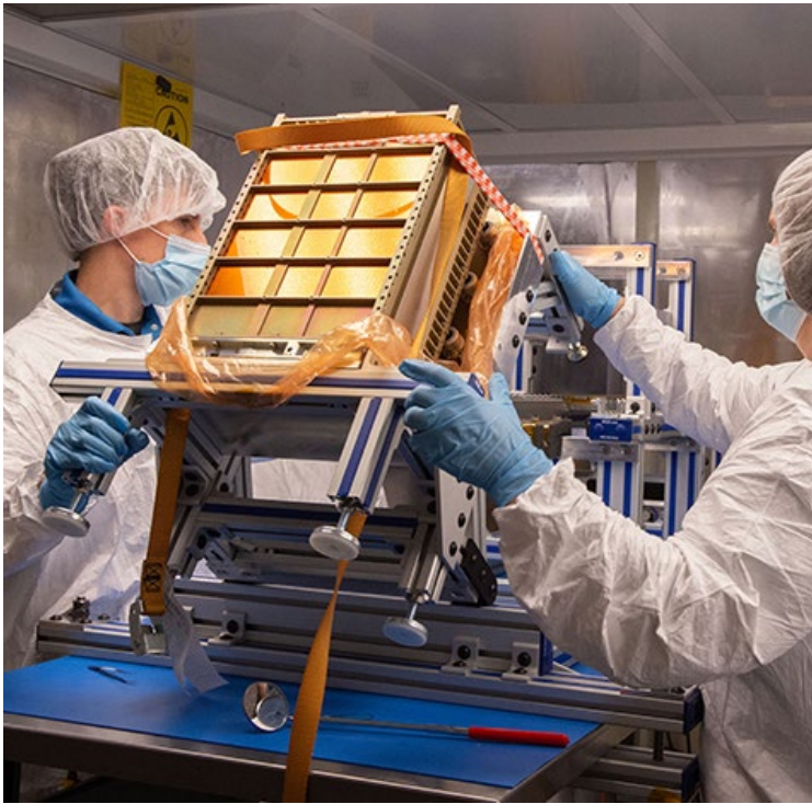
The NEA Scout CubeSat payload is integrated into its dispenser prior to the Artemis I flight.
