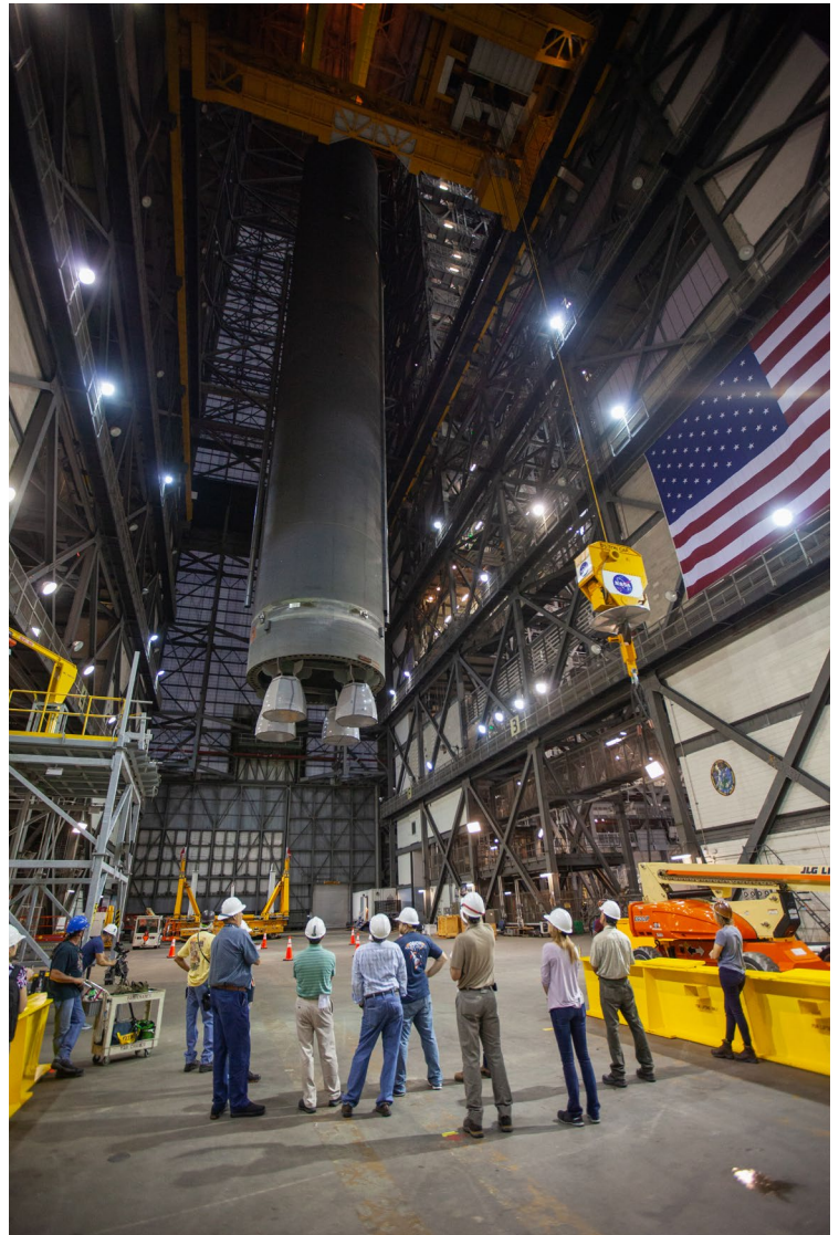
Engineers and technicians at Kennedy used the 212-ft. (65 m) pathfinder core stage simulator to practice lifts and moves in the Vehicle Assembly Building.
