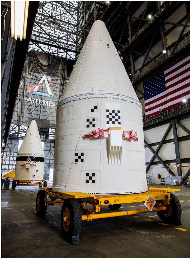
The forward assemblies for the SLS solid rocket boosters include aerodynamic nose cones, frustums, and forward skirts containing avionics.
