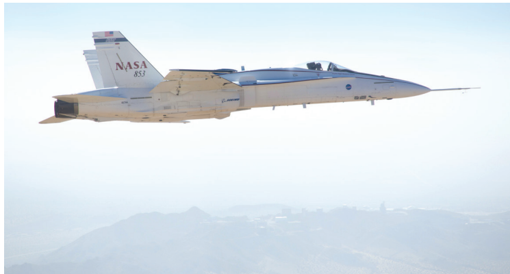
In 2013, NASA conducted a series of F/A-18 research flights to test SLS prototype software, including the previously adaptive augmenting control component. Adaptive augmenting control benefits total attitude control and increases flight control system performance when excessive tracking error is present and decreases responsiveness to undesirable frequency content. It expands the envelope under which the flight control system is capable of safely flying the vehicle.
