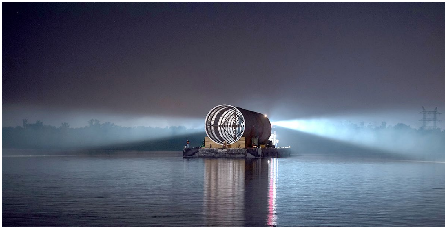
The core stage pathfinder mimics the structure of the SLS core stage, providing transportation, logistics, and lifting crews with the opportunity to rehearse with full-scale hardware before handling one-of-a-kind flight hardware.
