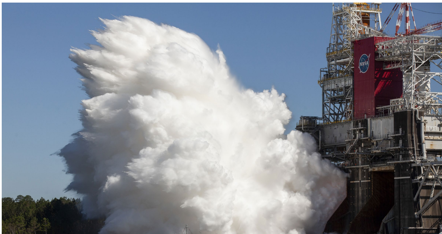
Eight major "Green Run" tests at Stennis of the Artemis I core stage and RS-25 engines culminated in a full-duration hot firing, the largest test of liquid-fueled engines since the Apollo Program.
