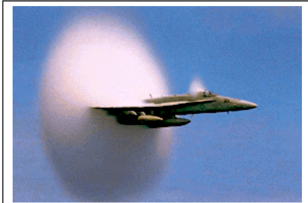
Spectacular photo of a fighter jet breaking the 'sound barrier' at a speed of 741 mph or 331 meters/sec (Courtesy Ensign John Gay).
