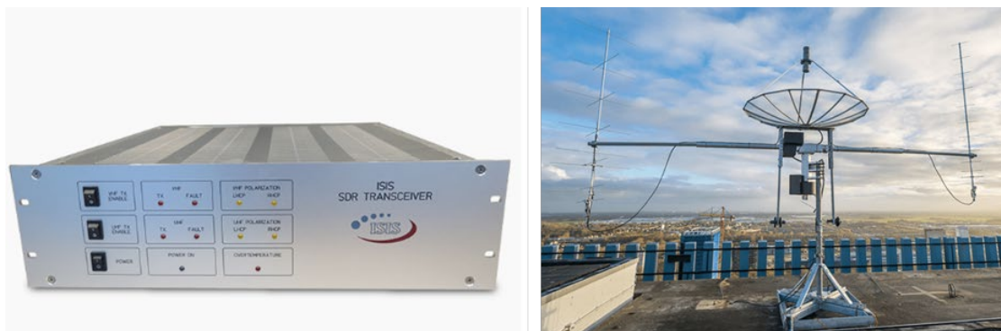
Figure 11.23: (left) ISISPACE ground station hardware, transceiver rack and tracking antenna (right). Credit: ISISPACE.
