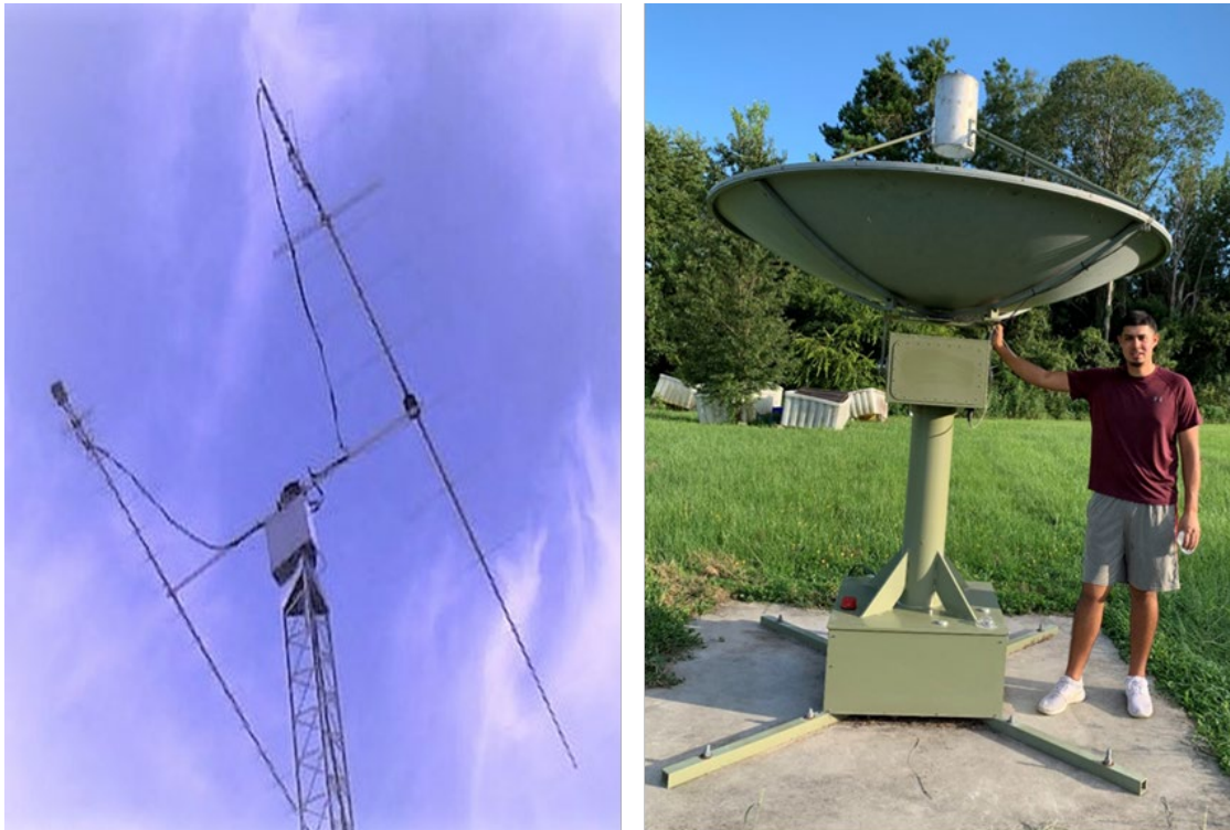
Figure 11.4: (left) The California State University Northridge Yagi ground station at 437 MHz and (right) The Aerospace Corporation parabolic dish ground station in Florida at 915 MHz. Credit: California State University of California, Northridge.
