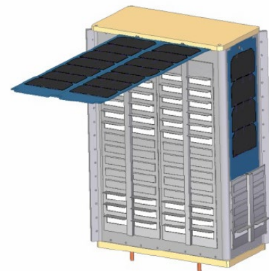
Figure 7.10: Passive Thermal Louver on 6U CubeSat Dellinger. Credit: NASA GSFC.
