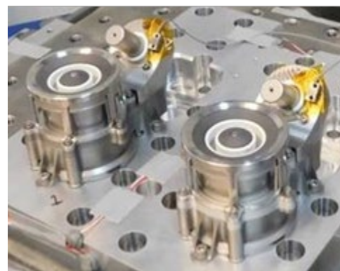
Figure 4.42: Two flight Aurora HETs undergoing qualification testing. Credit: Orbion Space Technology.
