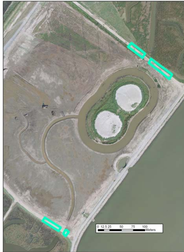
Figure 6. Aerial photo of the cross dikes between Cells 1A/B and B/C (still under construction) highlighting potential nesting areas that could be expanded and maintained vegetation free with minimal danger of erosion.
