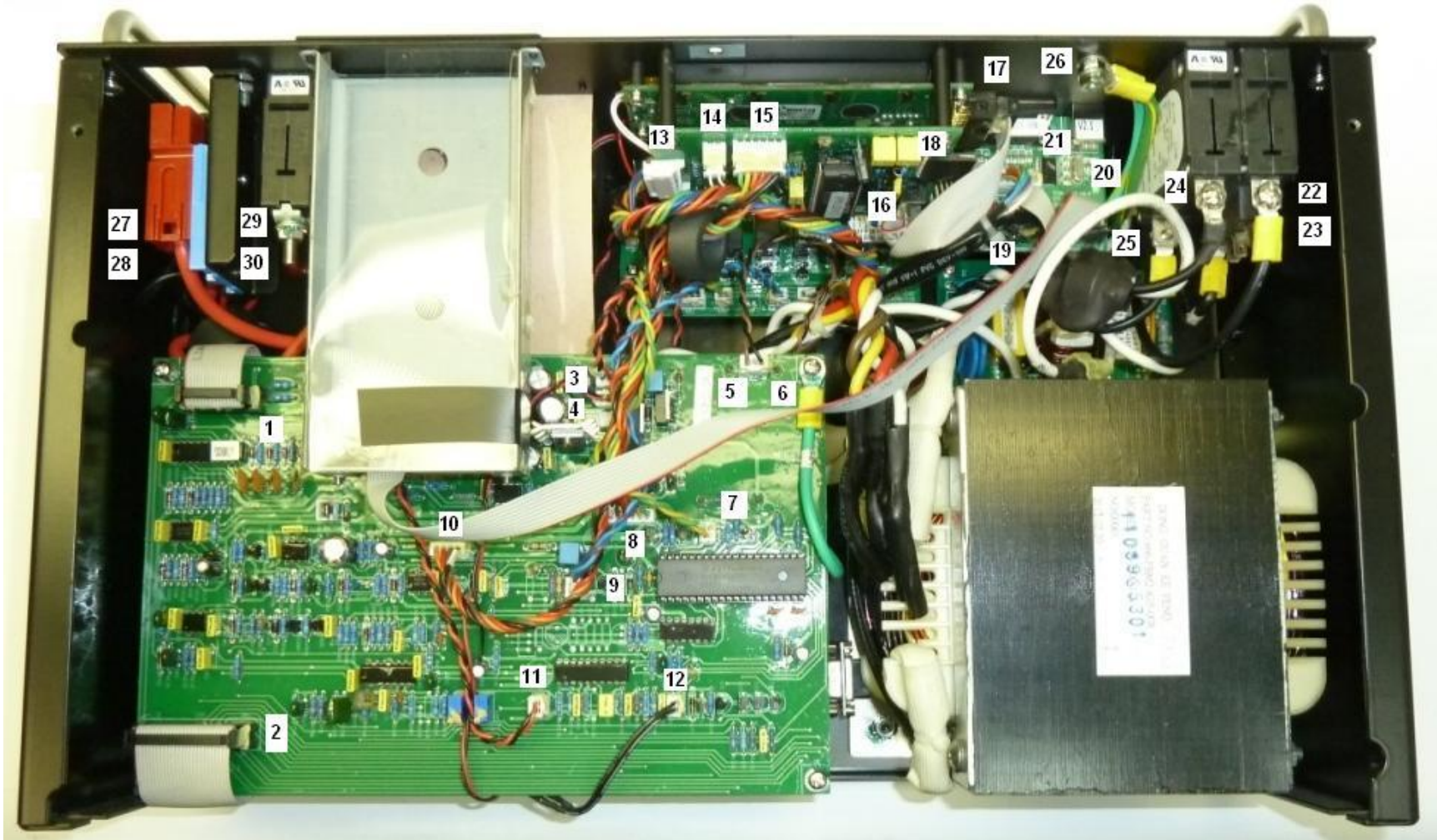
MP2000E Top Interior Connections
