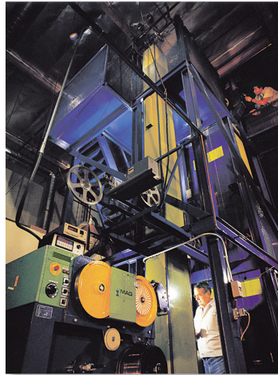
A MAG vertical oven enamel coats round, square and rectangular wire and is suitable for both small quantity and high production runs.
