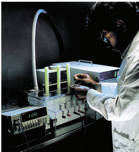
This Techné temperature-controlled bath provides MWS the capability to perform temperature coefficient of resistance (TCR) measurements for a variety of specialty metals and alloys. Precise resistance values can be obtained between -0°C and 100°C.
