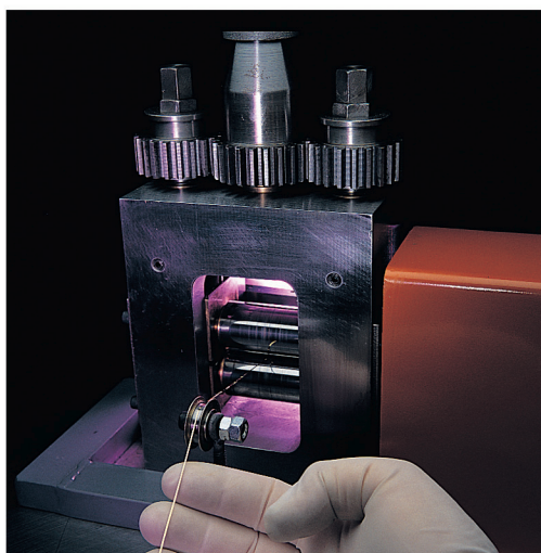
Precious metal rolling mill custom-built and specifically designed for fabrication of gold, silver, and platinum ribbon. Dimensional tolerances as tight as .00015".
