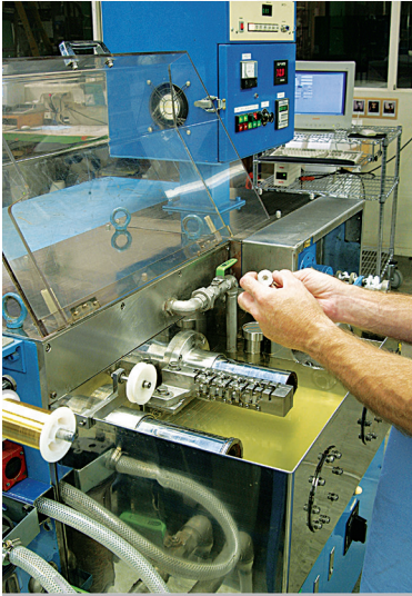
This specially designed machine draws precious metals to ultra-fine sizes in standard and custom diameters and temps.
