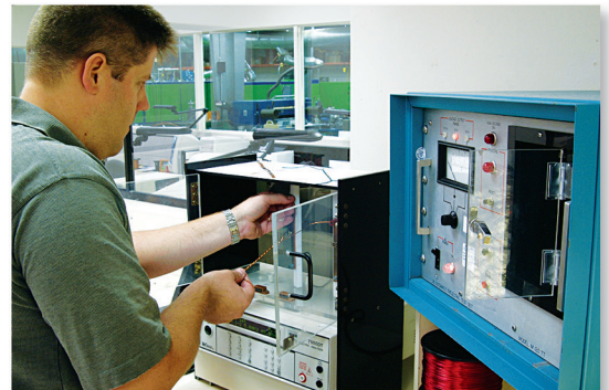
The Associated Research Model 7550DT Hi-pot/Dielectric tester has a testing range of 0 to 5,000 volts AC and 6,000 volts DC. The Hipotronics Model M 120 TT dielectric tester (shown right) has a range of 20,000 volts AC.
