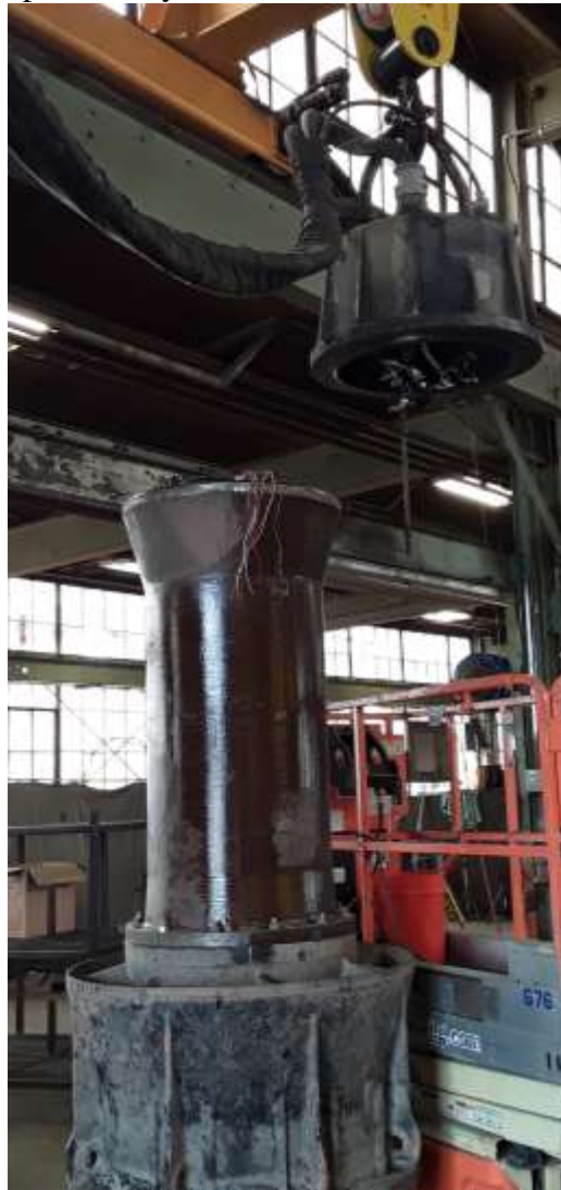
Installed upper cord cap assembly.
