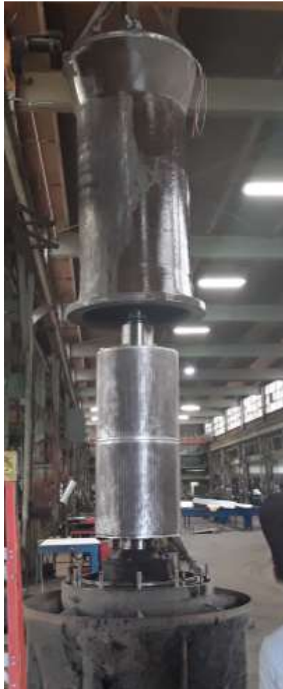
Lowering stator onto rotor and then assembled onto pump.
