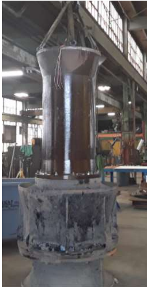
Lowering stator onto rotor and then assembled onto pump.
