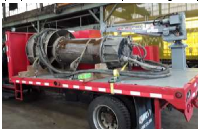
Cables wired and pump loaded onto truck to transport to testing facility.
