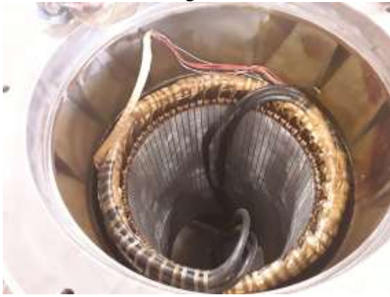
New stator in housing and lower sensor wiring.
