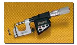
Interchangeable anvil micrometer permits quick, accurate measurements of tubing, cylindrical walls, from a hole or slot to an edge, and in many other hard-to-reach places. Two anvils are furnished with the tool – a round anvil, approximately .120" diameter; and a flat anvil, approximately .125" diameter and .060" in thickness. Anvils are rigidly held in a vise-type frame that allows for quick changes by a single lock screw.
