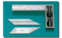
Double squares are popular with machinists, tool and pattern makers. Hardened, sliding blades are adjustable for a wide variety of uses. Faces of head are ground square. 6"/150mm size is equipped with a level, head is approximately 3-1/2" (90mm) long, and the faces approximately 9/16" (14mm) wide.
