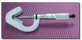
For checking out-of-roundness in centerless grinding and other machining operations; also for measuring odd-fluted taps, milling cutters, reamers. Direct reading. Carbide facings on spindle and anvils. Anvils match index of cutter teeth. Hardened, ground-from-the-solid spindle threads for accurate reading. No glare satin chrome finish. Quick-reading – every thousandth numbered.
