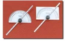
Combining protractor head graduated from 0 to 180 degrees in opposite directions with 6 inch blade graduated one side in 32nds and on reverse side in 64ths. Blade adjusts to any angle and may be clamped anywhere along its length by knurled thumb nut. Flat surface on back of the head permits laying tool flat on paper or work.
