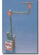
The very sensitive fine-adjustment is located on the magnetic base to eliminate indicator deflection when it is being adjusted.
