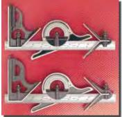
With reversible lock bolts, scriber, spirit level in both square head and protractor head. Direct reading double 180° protractor scale, and hardened steel machine-divided blade. Cast Iron Heads with black wrinkle finish.
