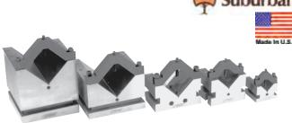
All vee blocks are parallel, square and central within .0002". Each block comes with one clamp and blocks are available in matched pairs. All models are made of hardened steel. Sizes other than those listed are available by special order.
