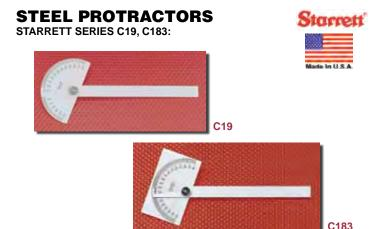
Useful for setting bevels, transferring angles and as small T-square. Graduated 0 to 180 degrees both directions. Six inch blade may be locked in position by tightening knurled nut. Flat back allows use for drafting. Satin Chrome finish.
