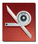
Any angle up to 360° can be laid out, or measured to 5 minutes or 1/12 degree with this tool. Acute angle attachment for measuring or laying out small angles furnished with tool. One side of tool flat which permits laying flat on work or paper. Satin Chrome finish. Fitted case.
