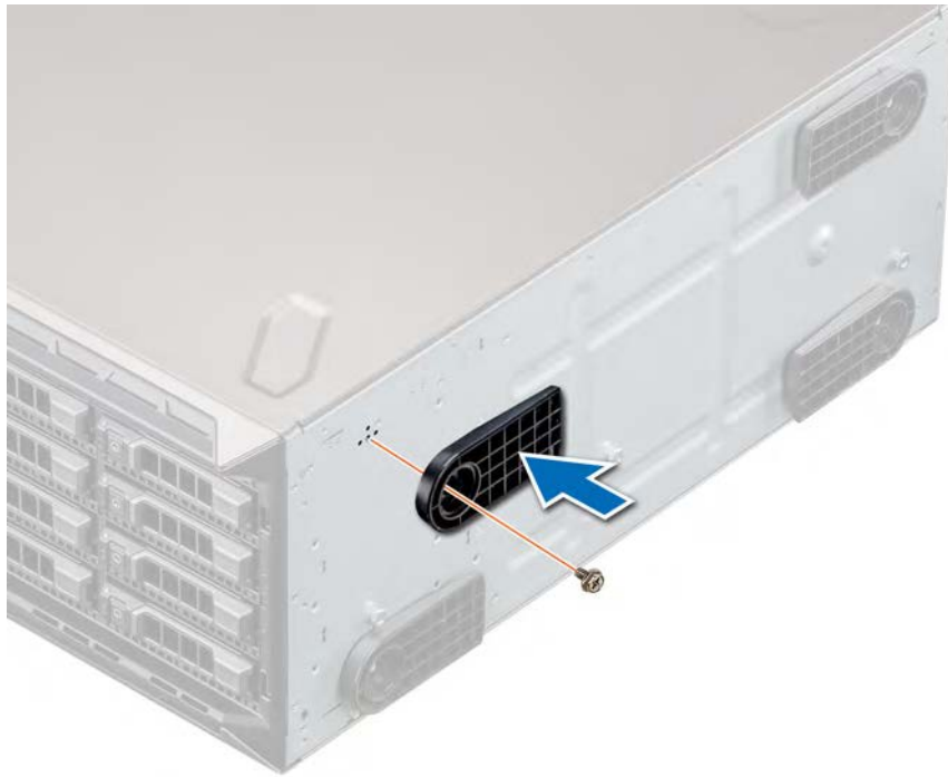
Figure 20. Installing the system feet
