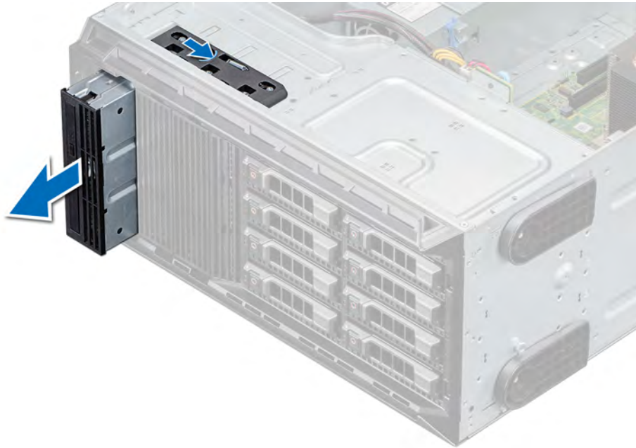
Figure 40. Removing the optical drive
