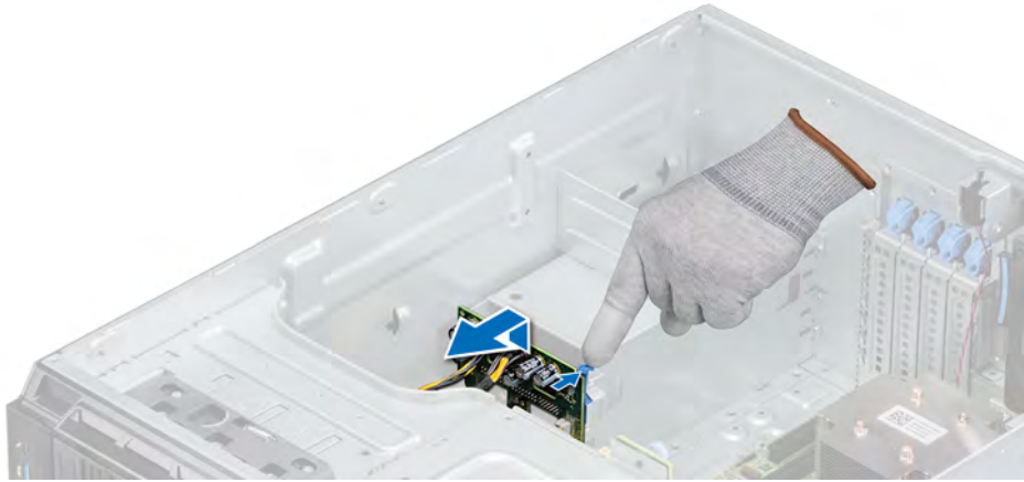
Figure 76. Removing the power interposer board
