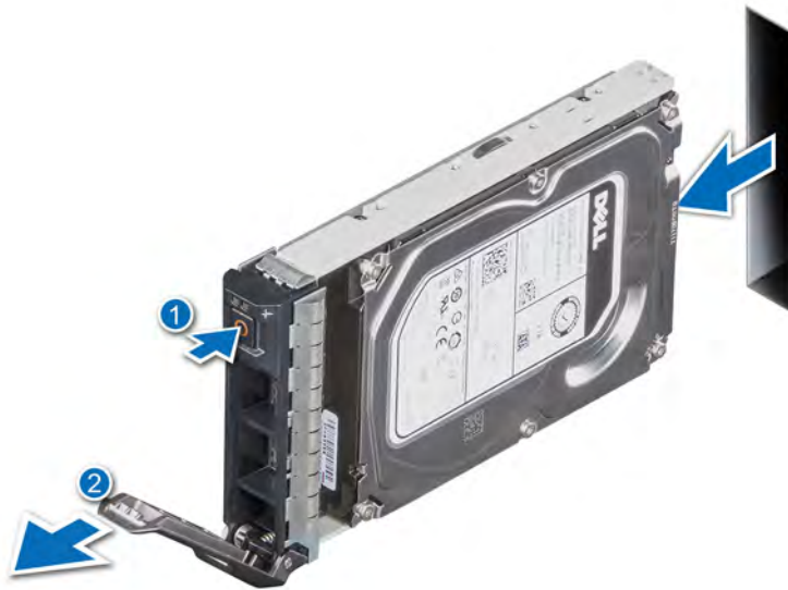
Figure 30. Removing a drive carrier
