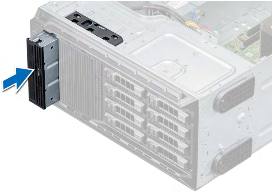
Figure 41. Installing the optical drive
