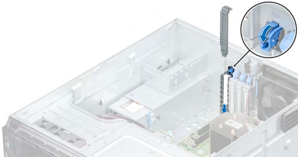
Figure 59. Installing the filler bracket
