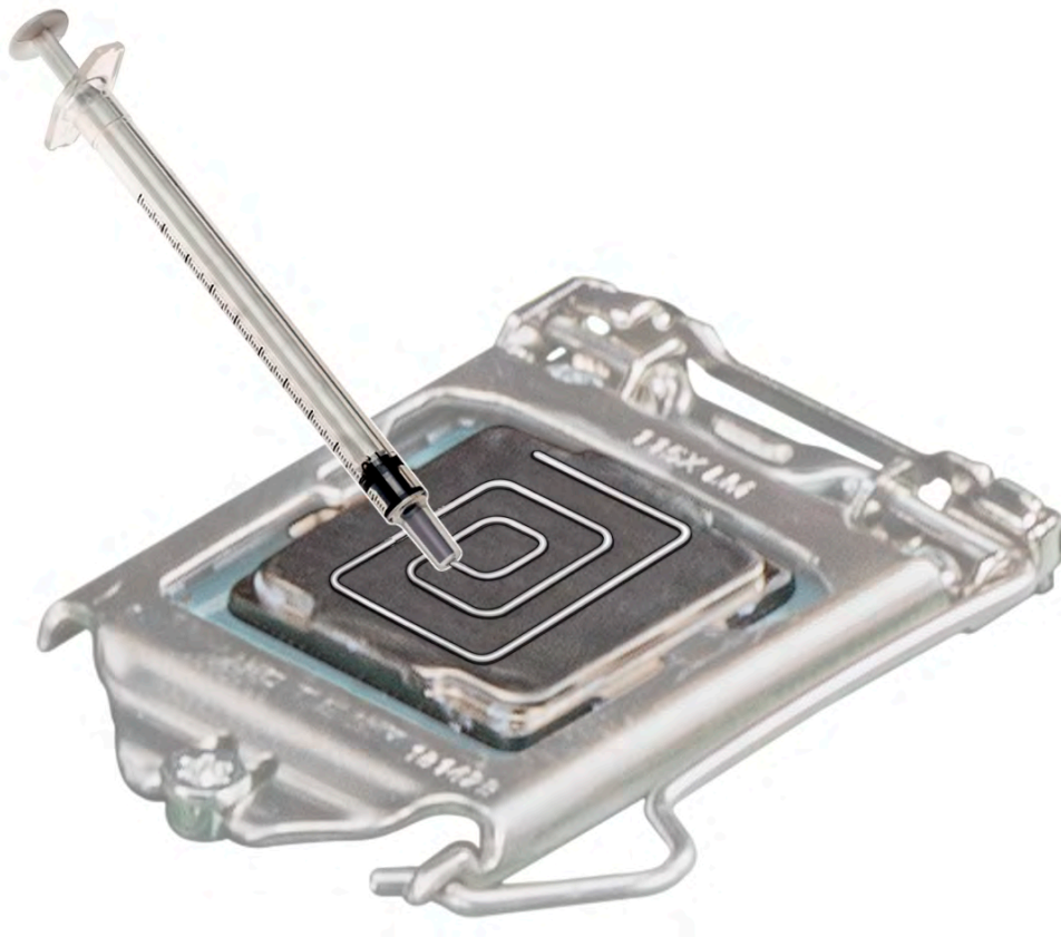
Figure 68. Applying thermal grease on top of the processor
