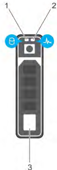
Figure 92. Drive indicators on the drive and the mid drive tray backplane
