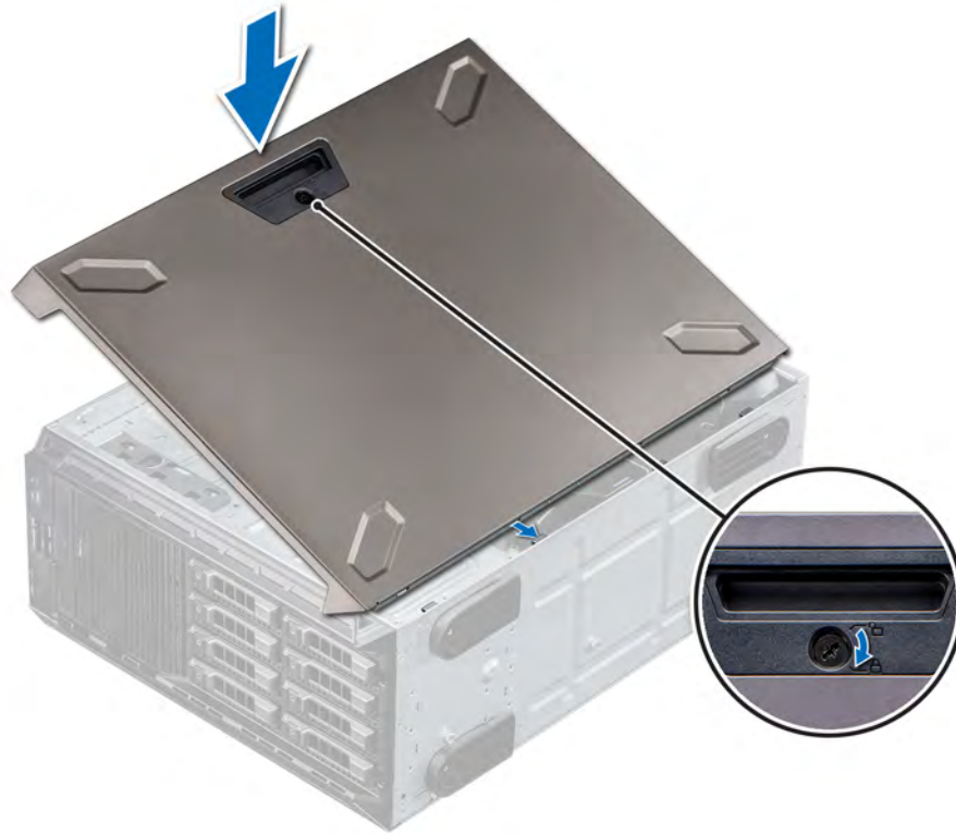
Figure 23. Installing the system cover
