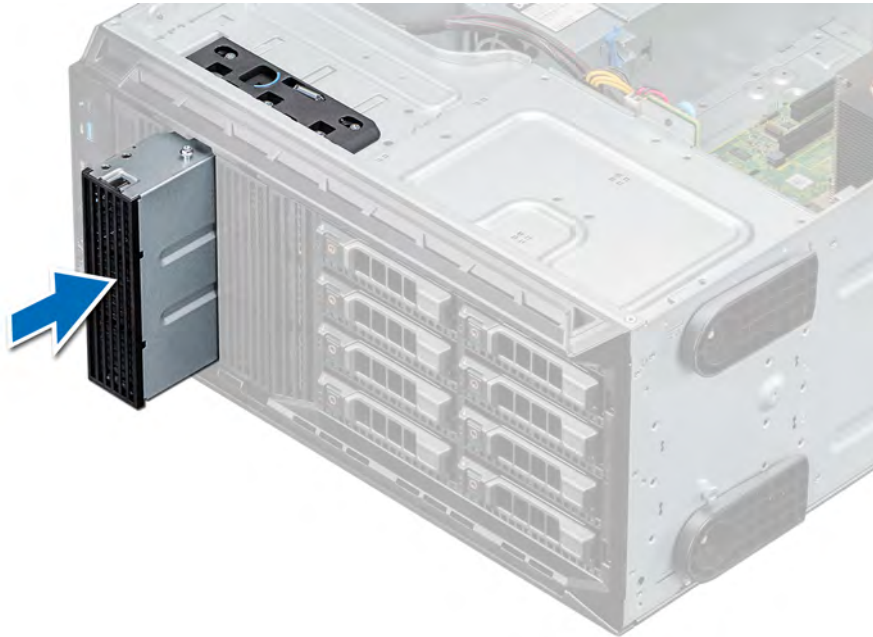
Figure 39. Installing the optical or tape drive blank
