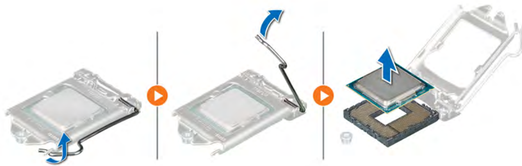
Figure 66. Removing the processor
