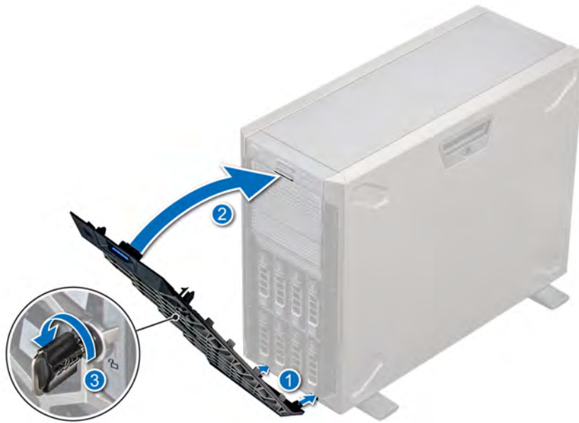
Figure 18. Installing the front bezel
