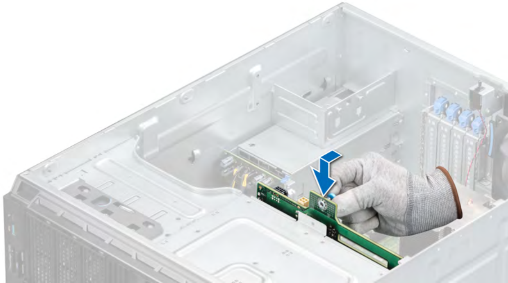
Figure 46. Installing the drive backplane
