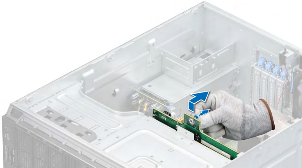
Figure 45. Removing the drive backplane
