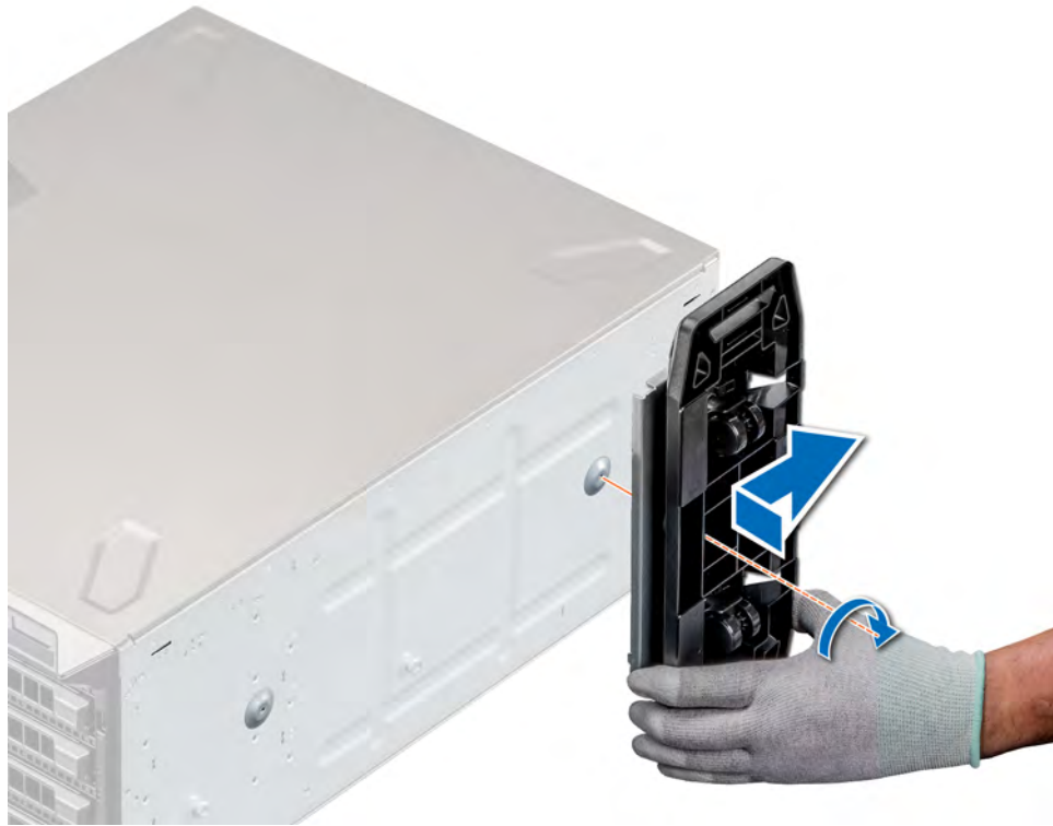
Figure 21. Installing castor wheels
