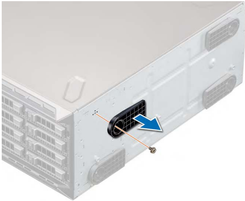
Figure 19. Removing the system feet
