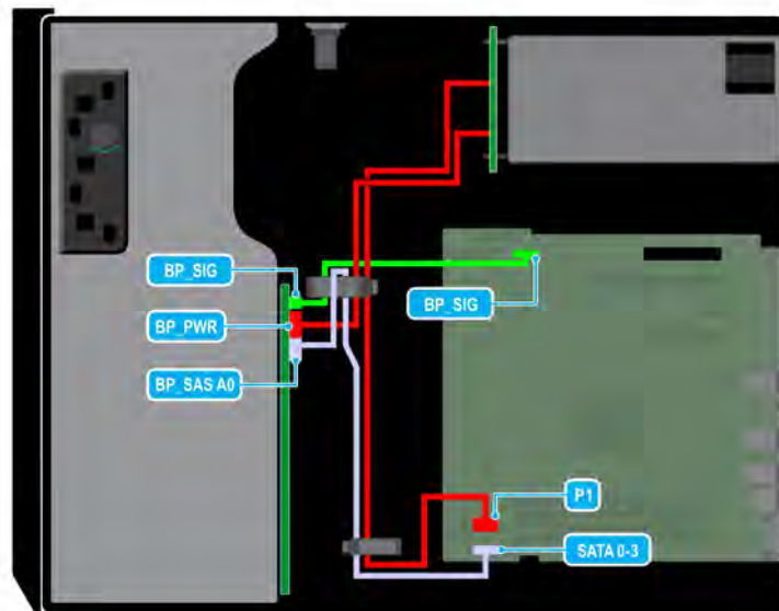
Figure 47. Cable routing - 8 x 3.5-inch, SATA drive backplane
