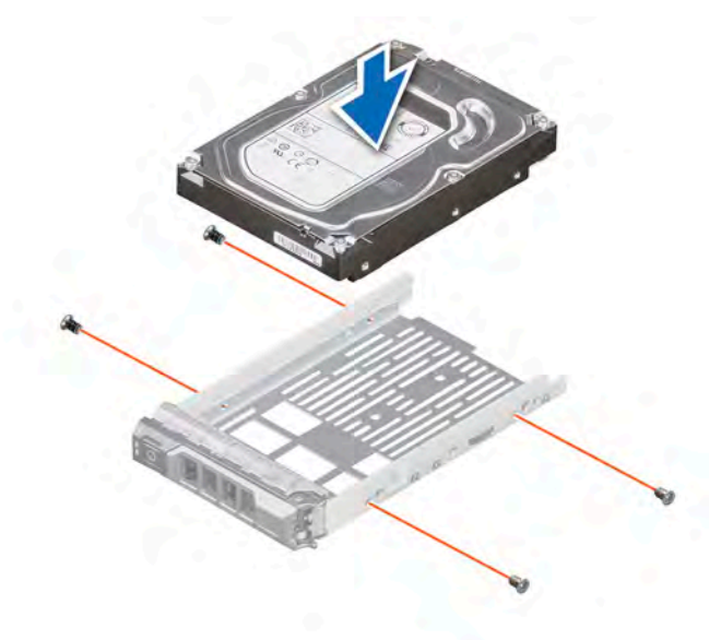
Figure 33. Installing a drive into the drive carrier
