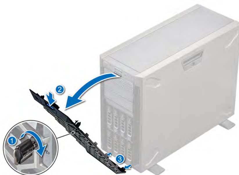
Figure 17. Removing the front bezel
