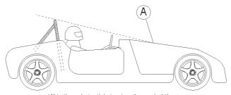
'A' is the substantial structure forward of the driver such as to act as the front rollbar. No part of the driver's helmet is to pass through a line struck from the top of the rollbar to this structure.
