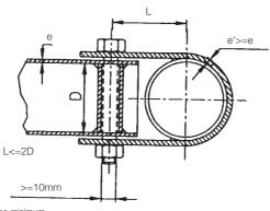
L must be minimum The clamp width must be at least 25mm
