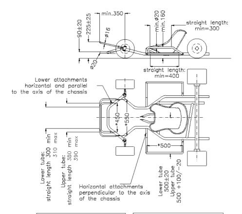
Lower Tube Ø 20mm with one constant radius.
