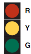
Figure 49 - Signal Section used with a shared lane that has no turning movement controls. Source: MD-MUTCD
