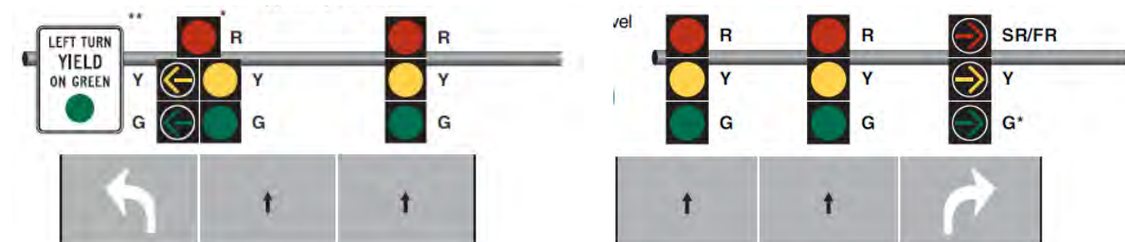
Figure 52 - Typical Positions and Arrangements of Signal Faces for Exclusive/Permissive Turn Modes. Source: MD-MUTCD
