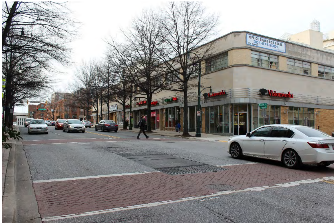
Figure 15 - Fenton Street at Roeder Road, looking northbound. Pedestrians are susceptible to the multiple-threat at this intersection. MCDOT is planning to implement a pedestrian hybrid beacon (HAWK) signal here.
