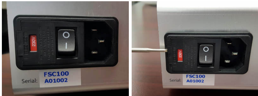
Figure D.2: To change fuse or voltage, open the fuse cartridge cover with a screwdriver inserted into a small slot at the left edge of the cover, just to the left of the red voltage indicator.
