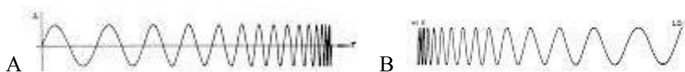
Figure 5.4: A. Upsweep - the frequency increases with time; B. Downsweep - the frequency decreases with time.
