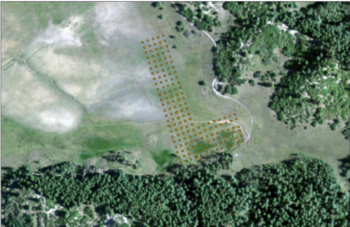
Figure 9.19: The location of the EM grid in Shahan's map is shown above. The processed data does not include the portion that extends west. The processed data only extends 40m west and then extends north from there.
