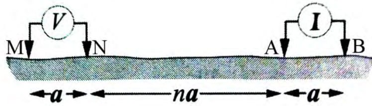
Figure F.5: Dipole-Dipole array layout [72]
