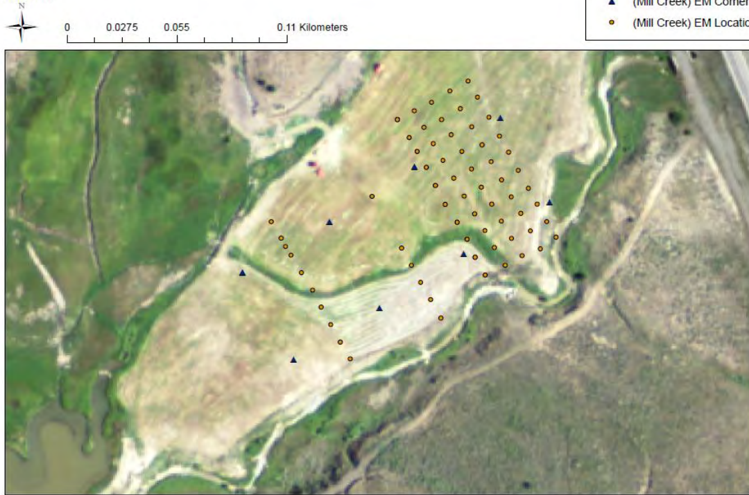
Figure 9.6: Shows the GPS locations of the EM57 grid and the EM47 lines at Mill Creek near the highway (Highway 84 is on the right side of the image).
