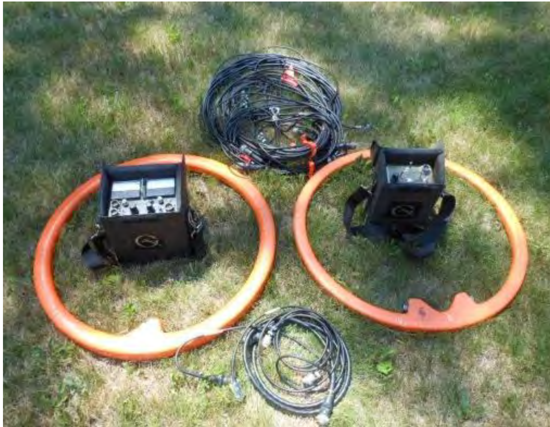
Figure E.3: A picture showing all of the EM34 components laid on the ground.
