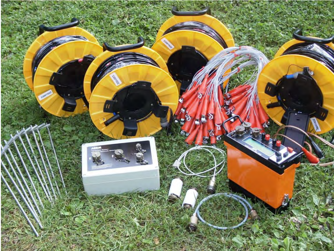
Figure F.2: ABEM (orange) with cables, electrodes, cable connectors, and flags
