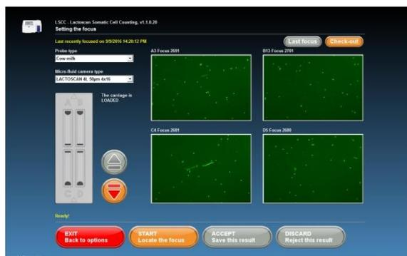
The device takes the cartridge in and focusing can be started.
