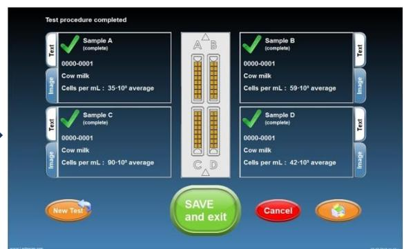
LACTOSCAN SCC performs the test and gives final result. The final result is an automatically calculated average result from the results of the tests of chambers A, B, C, D.
