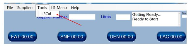
It opens the software tool for calibration. The operator chooses the Com Port, and presses the button Start. After that inputs the parameter values in the fields. With the button Measure starts a new measurement of the sample in calibration mode.
