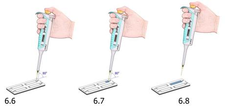
In order to load the rest of the micro-fluidic cameras of the LACTOCHIP x4 / LACTOCHIP x2, repeat the procedure described in points 1 to 6 by consecutively filling the micro-fluidic cameras from A-D.
