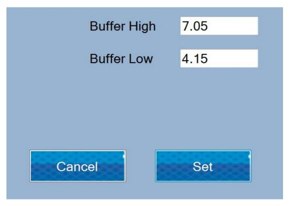
The operator inputs the values of the buffers used for calibration. Selection of buffers and principles of work with the pH meter are described in the document WLS-TechManual. By pressing the Set button to go to the actual calibration. Reports of this process is displayed in the System Status, in the upper right corner of the screen. By pressing the Cancel button procedure is terminated and transferred to the main screen.
