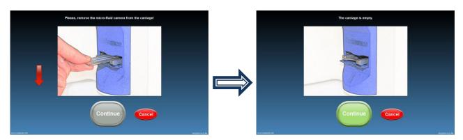
6. Press . The software prompts for placing the LACTOCHIP with the samples for which data are entered.
