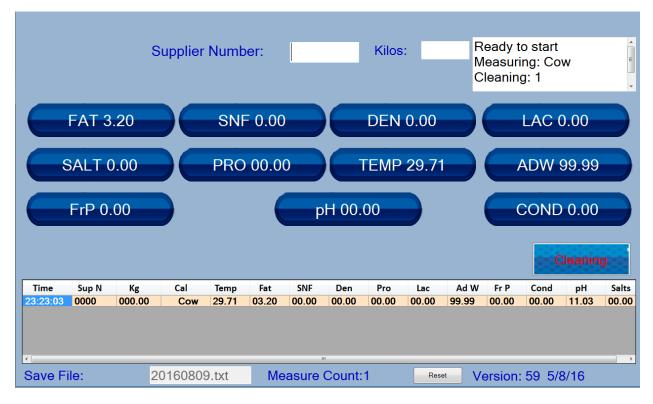
After the cleaning cycles are finished, the analyser returns "Lactoscan Cleaned" message and "Ready to start"
