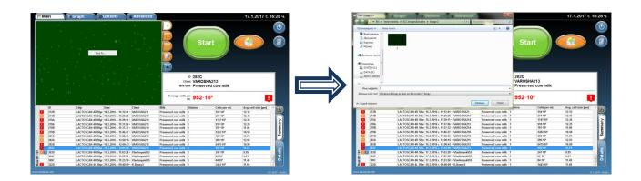
3. Select the folder where you want to save the image, write the name of the image, select the .BMP file format from the dropdown menu and press button SAVE to finally save the image as .BMP file.
