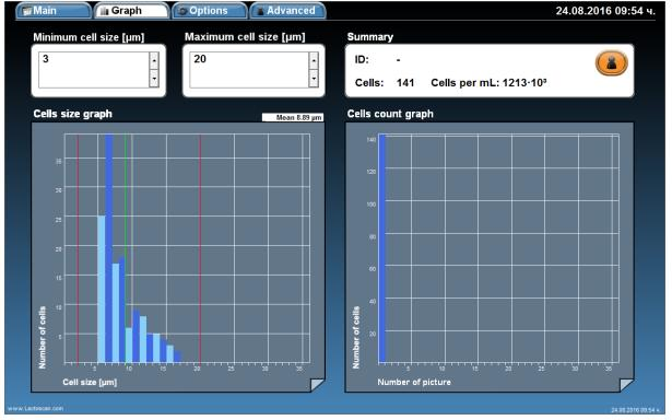
When the cell size range is set from 3 to 20  $\mu$ m, the counted cells are 141, equivalent to  $1213 \times 10^3$  cell/mL. The cells size is between 6 and 17  $\mu$ m. The average cell size is 8.89  $\mu$ m. Most of the cells are with size 6-11  $\mu$ m. The cell size peak is at 7  $\mu$ m.
