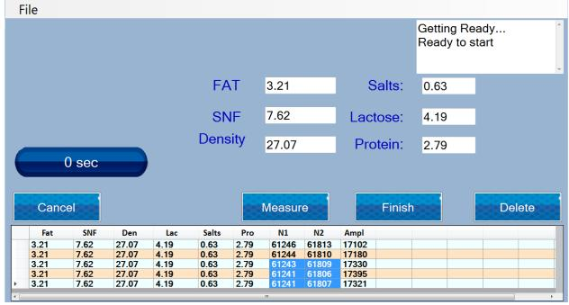
If results for N1 and N2 are with bigger difference than 3x, check milk's acidity (it has to be normal one); stir the sample and measure once again 5 times; in case you receive again not stable results, address our service.
