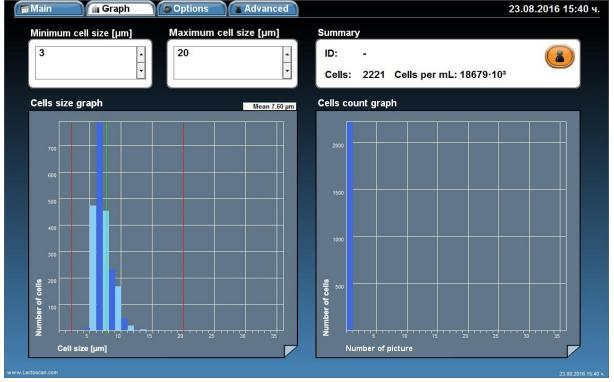
When the cell size range is set from 3 to 20  $\mu m$ , the counted cells are 2221, equivalent to  $18679 x 10^3$  cell/mL. The cells size is between 5 and 14  $\mu m$ . The average cell size is 7.60  $\mu m$ . Most of the cells are with size 6-8  $\mu m$ . The cell size peak is at 7  $\mu m$ .
