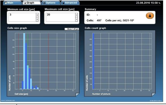
© 2021 "Milkotronic"Ltd All rightsreserved When the cell size range is set from 3 to 20  $\mu$ m, the counted cells are 497, equivalent to  $5021 \times 10^3$ . The cells size is between 4 and 15  $\mu$ m. The average cell size is 7.48  $\mu$ m. Most of the cells are with size under 9  $\mu$ m. The cell size peak is at 7  $\mu$ m.
