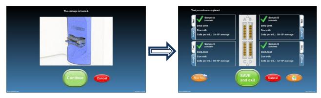
LACTOSCAN SCC performs the test and gives final result. The final result is an automatically calculated average result from the results of the tests of chambers A, B, C, D.
