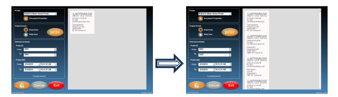
5. If printing the results from the analysis, made for a certain period of time is needed, then, with the assistance of a calendar the initial and the final date of the period can be set.
