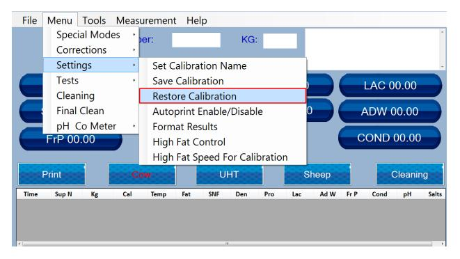
This way the user can have any number of calibrations saved to the tablet and when needed Restore(replace) one calibration with another
