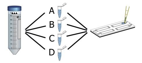
• After sample preparation take  $100\mu$ L of sample and put it into an eppendorf tube. Do this a total of 4 times for the 4 cameras of the chip.
