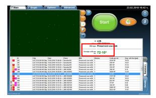
Setting the limits of the subclinical mastitis is made by changing the value in the field "Warning level of cells count". Changing of the value is made with up and down arrows or by setting the value manually.
