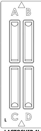
**LACTOCHIP x4** has four separate closed chambers (A, B, C  $\mu$  D), that allow analysis of four different samples. Each chamber's capacity is 8  $\mu$ L. LACTOSCAN SCC makes 16 pictures of the sample in each chamber and then it performs the analysis via a specific algorithm.
