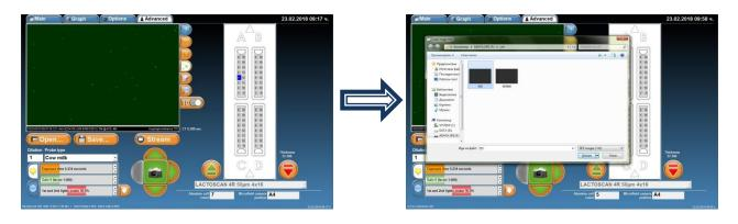
13. Button Stream – after pressing the button Stream, mode Movie is activated and LACTOSCAN SCC starts making consecutive pictures as the time for changing the image depends on the set exposition time. For example, if it is set to 1.945 sec. exposition time, images on the display will be changed in approximately 1.945sec. Mode Movie is used when a number of sections of
