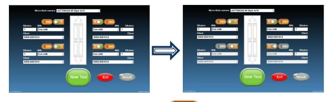
4. For a quick analysis, press button and select a test from the dropdown menu. You can select from test "Scanning 25% of positions", test Scanning 50% of positions", test "Scanning 100% of positions".
