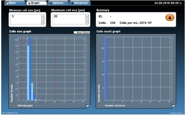
When the cell size range is set from 3 to 20  $\mu$ m, the counted cells are 238, equivalent to 2074x10<sup>3</sup> cell/mL. The cells size is between 5 and 13  $\mu$ m. The average cell size is 6.88  $\mu$ m. Most of the cells are with size under 9  $\mu$ m. The cell size peak is at 7  $\mu$ m.
