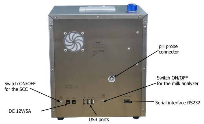
Switch ON/OFF for the SCC. It is used to power on / off the SCC part of the device.
