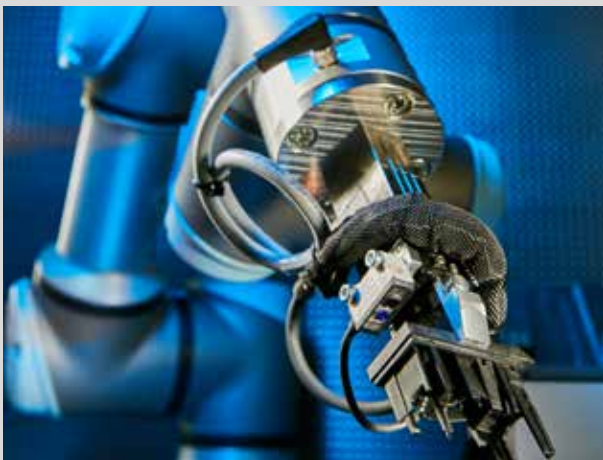
Distance measurement in robotics applications directly from the gripper
