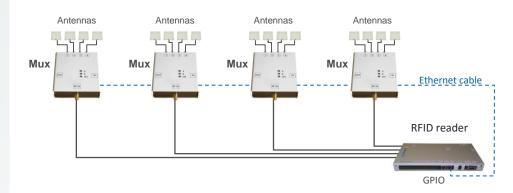
AdvanMux-4 can be controlled both by standard +5 V and open collector digital outputs.
