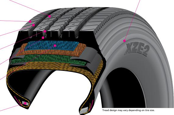
Rectangular bead bundle a Michelin exclusive – simulates a solid steel rod "strapping" the tire onto the wheel. This design stabilizes the entire bead region and minimizes fatigue in order to extend casing life.
