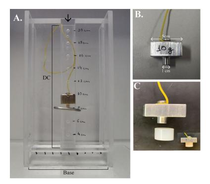
**Fig. 1** Spinal cord crush injury model. (a) Apparatus to control the drop height (indicated in cm on drop column). Arrow indicates original placement of the weight into the drop column (DC). (b) Approximate size of weight that fits into the drop column. (c) Plastic cap used on the weight to disperse the impact and prevent piercing through the tissue
