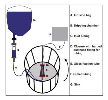
**Fig. 1** Overview of the OKR setup. The infusion bag (A) is connected to the dripping chamber (B), necessary to provide water to the fish via the inlet tubing (C). The fish is restrained inside a glass fixation tube (E), closed with barbed bulkhead fitting (D). Water will be discarded via the outlet tubing (F) in the sink (G)
