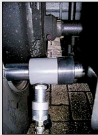
The Winntec Wheel Breaker Set in use.
