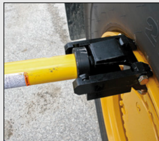
The Stinger Bead Breaker in use.
