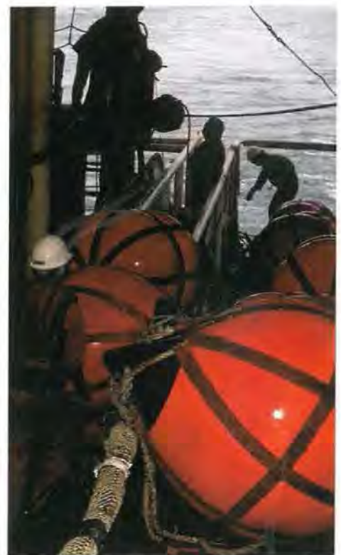
Crews recover air-gun floats during a seismic survey in Australia's Bass Strait. ExxonMobil's Geophysical Operations Group has completed seven years and 15 million project hours without an employee or contractor lost-time injury.
