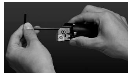
3. Tighten 3 bolts to attach the head
