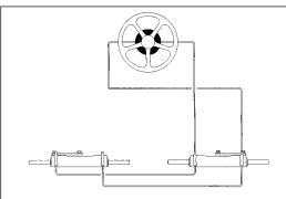
Dual engine dual cylinder application diagram
