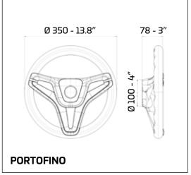
All PORTOFINO steering wheels are provided with an exclusive hub that easily allows the steering wheel to always be aligned properly.
