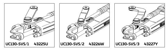
In the applications with dual UC130-SVS cylinder it is necessary to order a standard UC130-SVS cylinder (link arm attached to the starboard side of the cylinder) and a port UC130P-SVS cylinder (link arm attached to the port side of the cylinder). See appropriate section for A95 tie bar required for use on dual engine/dual cylinder applications.
