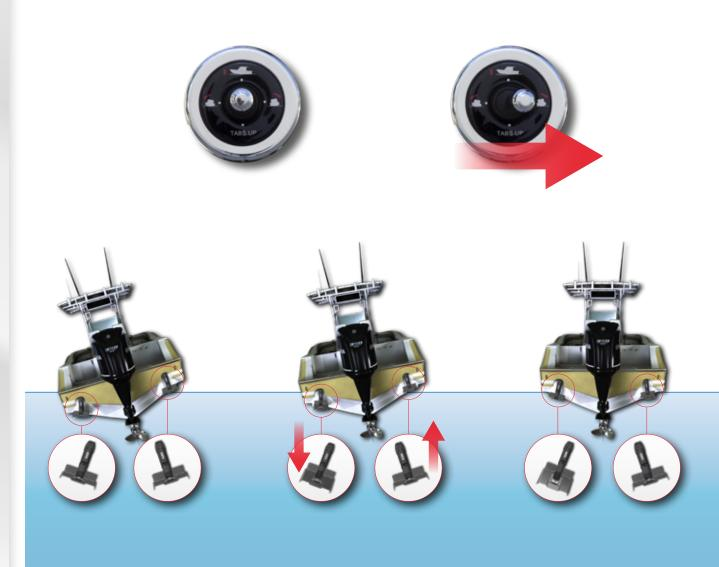
The unique profile of the Uflex planes offers greater efficiency and stern lift than traditional flat planes, often providing the opportunity to use a smaller size tab with the same performance of a larger flat plane.
