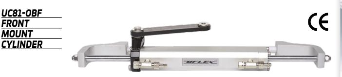
**UC81-OBF** - Balanced: the number of turns lock-to-lock is equal port to starboard and vice-versa. **Depending on the applications on the outboard engine, the UC81-OBF can be installed port or starboard**
