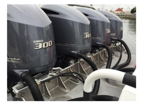
TIE BARS FOR TWIN OUTBOARD ENGINES
