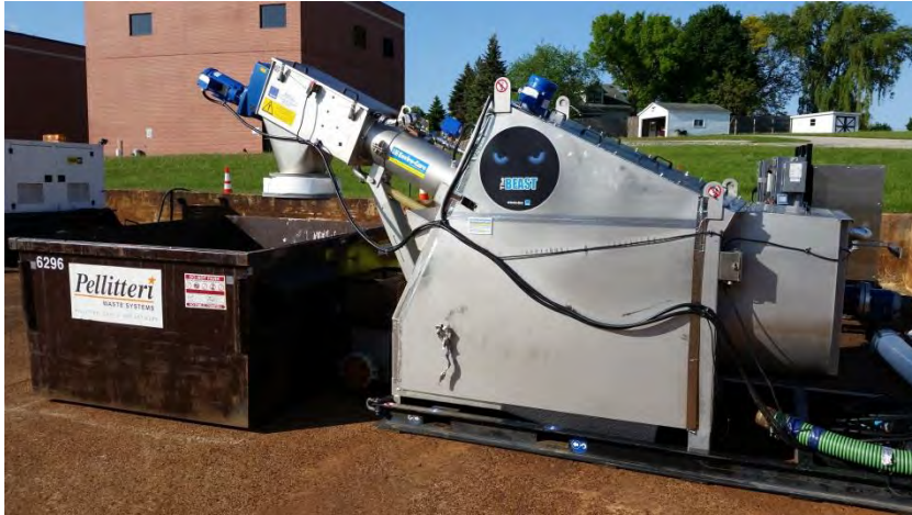
Figure 3 – Flo-beast Screening Skid
