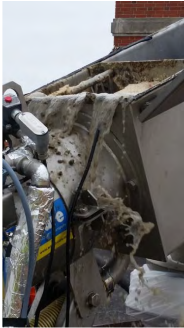
Figure 15 – Plug caused liquid to backup out of compaction zone
