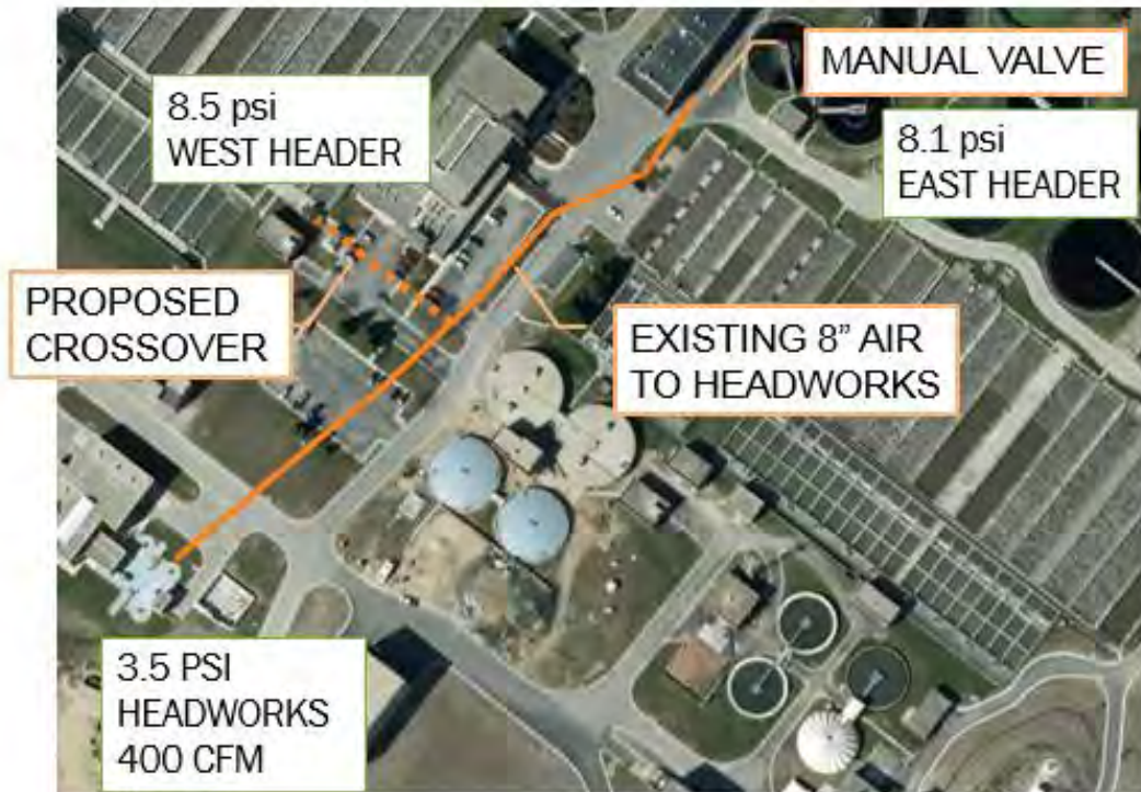
Figure 8-1. Possible east-west air piping connection
