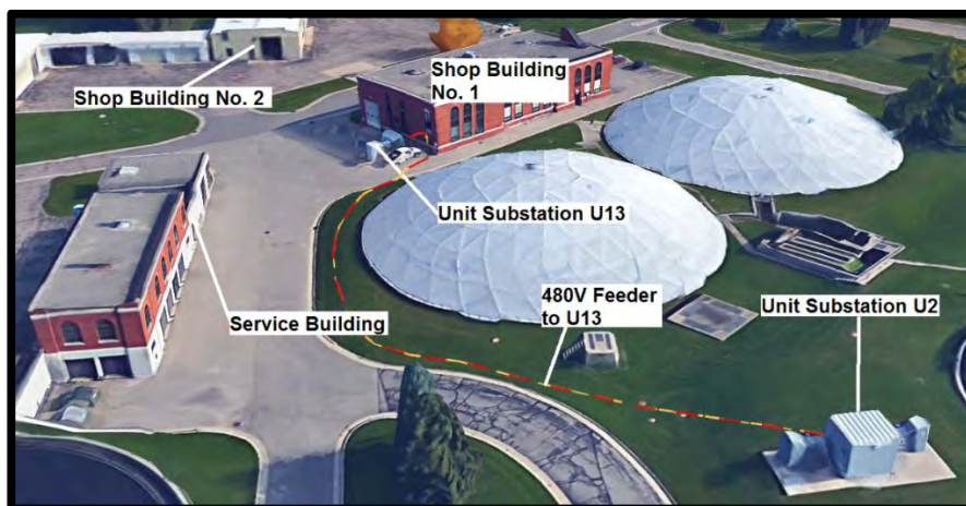
Figure 25–Unit Substation U13 Site Map
