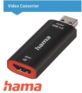
Video Recording Stick, USB Plug - HDMI™ Socket, 4K
